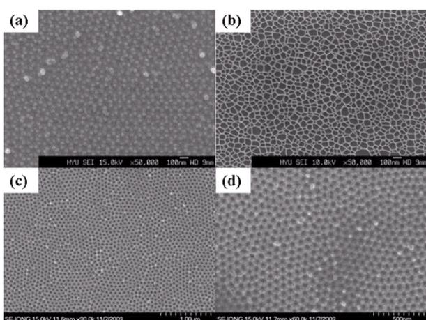
Fig. 2. SEM images of the AAO surfaces after first anodizing under different conditions: (a) 6.0 mA 10 h, and (b) 2.5 mA, 6 h. (c) and (d) show SEM images after second anodizing and widening in phosphoric acid at 30 °C, respectively.
