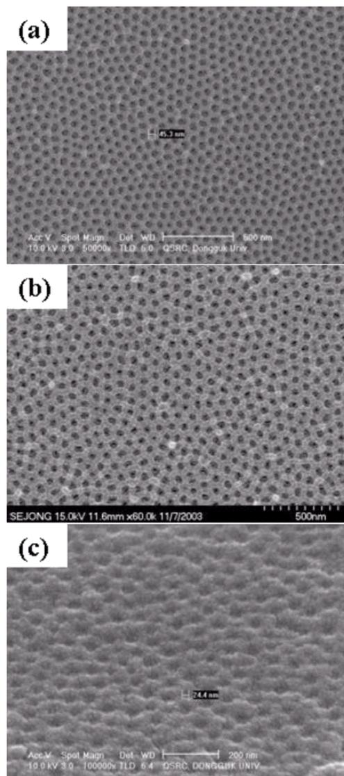
Fig. 3. SEM images of AAO templates prepared under different current conditions, with a constant bias voltage of 40 V and a time duration of 7 h: a) 40 V, 8 mA, 7 h ; (b) 40 V, 6 mA, 7 h; (c) 40 V, 4 mA, 7 h.
