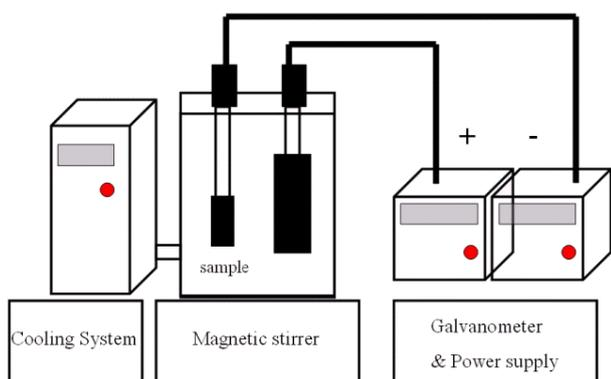
Fig. 1. Schematic diagram of AAO experiment equipment in current mode.
