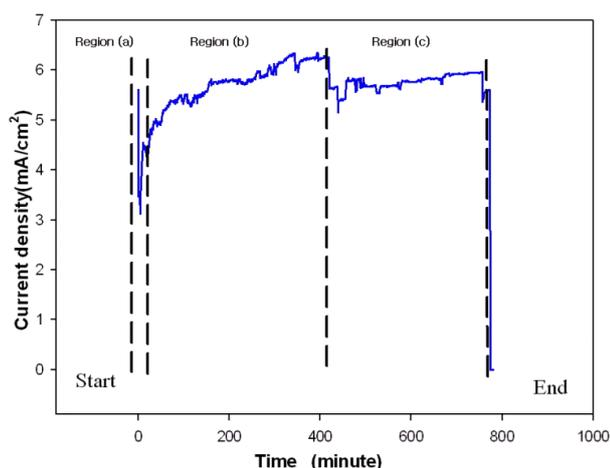
Fig. 4. Anodizing current density versus time, where the operation was done in current mode.
