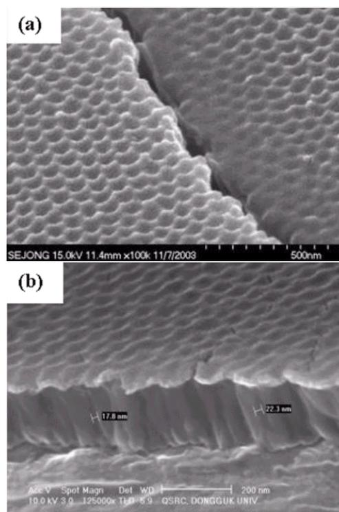
Fig. 5. (a) tilted and (b) cross-sectional SEM views of the AAO templates, to observe pore depth.
