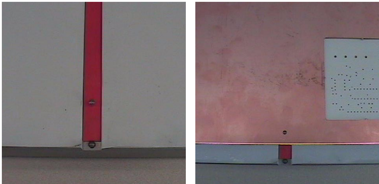
Figure 4.3: These photographs illustrate the retention pin mechanism used to ensure top-bottom registration of the circuit board during milling. The bed of the mill has a longitudinal groove into which two (red) plastic strips are inserted. A hole is drilled in each of these strips and a retention pin is inserted. The photograph on the left illustrates this arrangement. A circuit board must have holes drilled to accommodate the retention pins. The board is placed over these pins when milling, thus ensuring registration (see photograph on the right).
