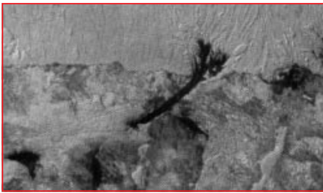
Fig. 3—This magnification of the new iron electroplate and cast iron interface shows the molecular bond of the plating to the basis metal. (Note flake of graphite extending into the electroplate.)
