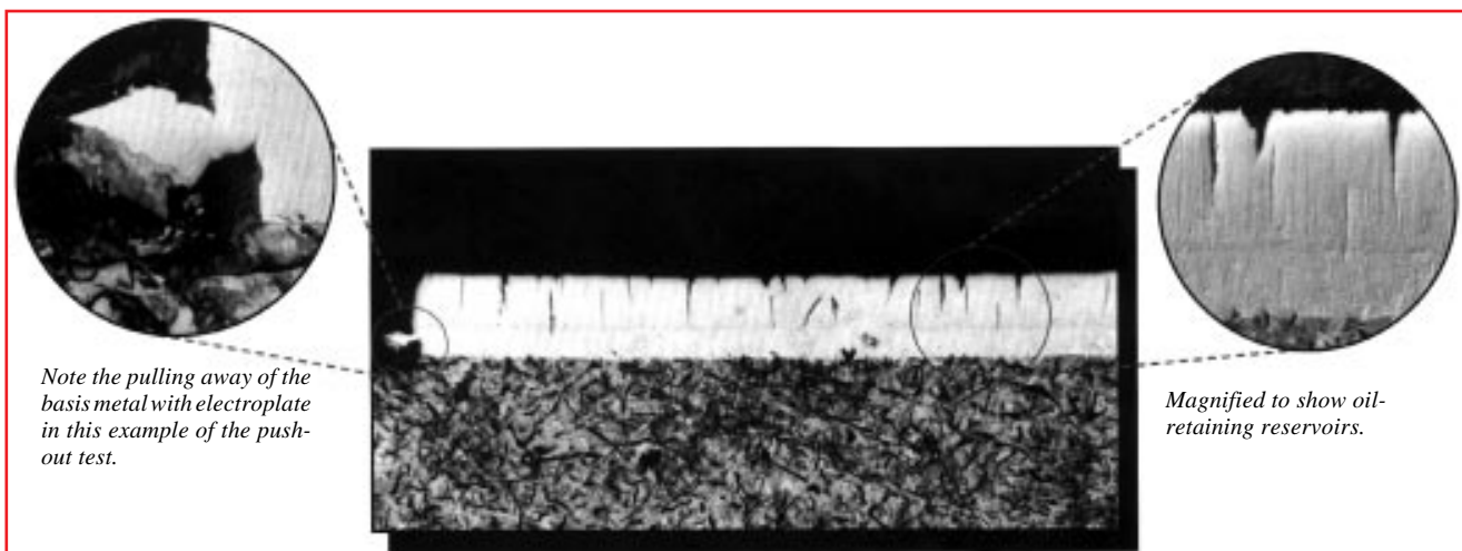
Fig. 2—A magnified cross section of a deposit on cast iron, and the results of a routine bond check.
