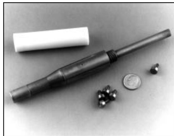
Fig. 3—Disassembled view of Rotating Disk Electrode and removable Rotating Disks.
