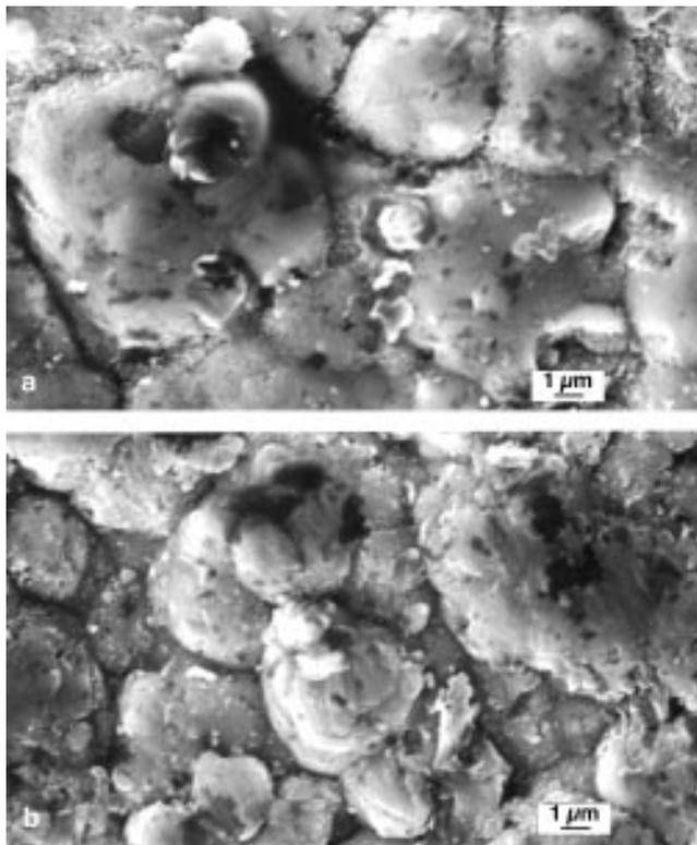
Fig. 1—Surface morphology of composite Cr-Ni-Al<sub>2</sub>O<sub>3</sub> deposit. Current density, 7A/dm<sup>2</sup>: (a) 47 and (b) 312 g/L alumina in electrolyte.
