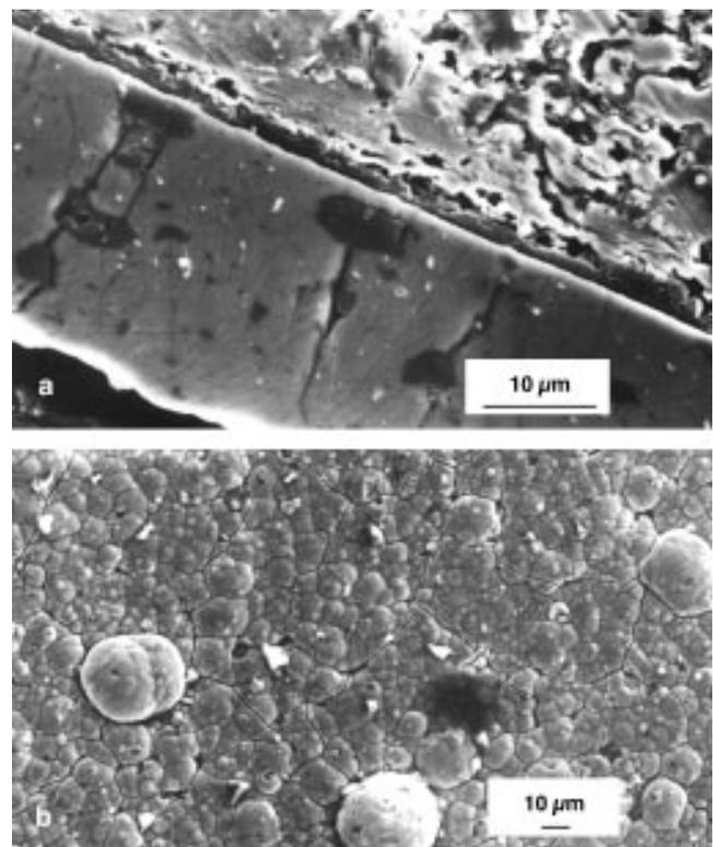
Fig. 2—Crack appearance by cross-section (a) and surface (b) examination. Current density, 21 A/dm<sup>2</sup>; Al<sub>2</sub>O<sub>3</sub> content of bath, 31 g/L.
