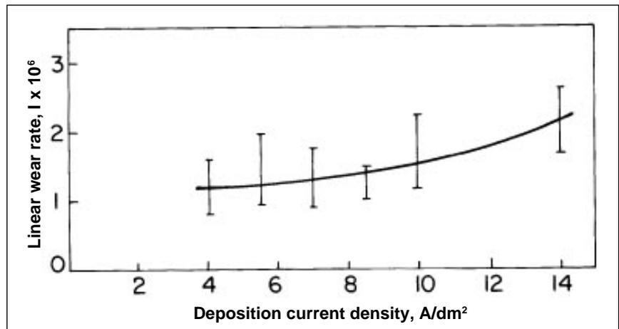
Fig. 7—Effect of current density on linear wear rate of Cr-Ni-Al<sub>2</sub>O<sub>3</sub> deposits with 75 g/L alumina powder in the electrolyte.
