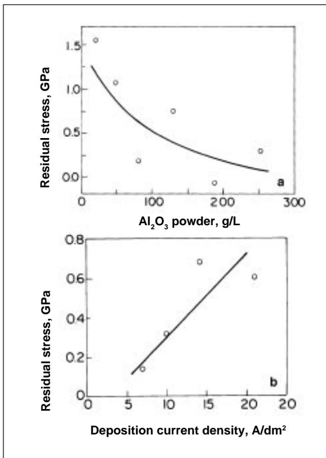
Fig. 8—Effect of current density (a) and amount of alumina powder in bath (b) on residual stresses in Cr-Ni-Al<sub>2</sub>O<sub>3</sub> deposits: (a) Al<sub>2</sub>O<sub>3</sub> in bath 75 g/L; (b) current density, 7 A/dm<sup>2</sup>.
