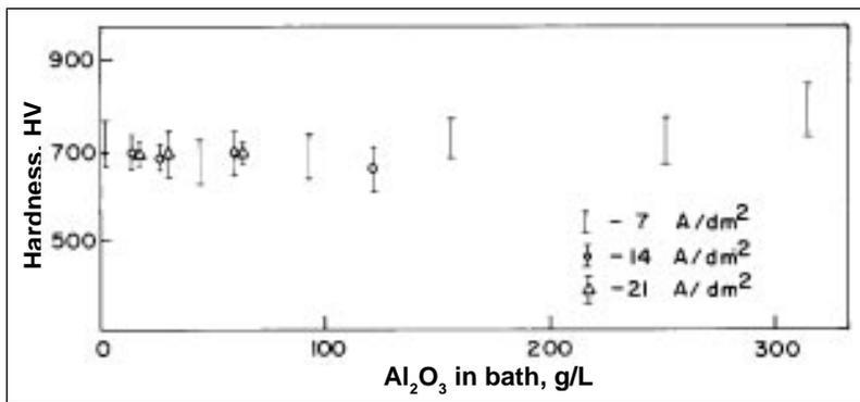
Fig. 3—Microhardness of Cr-Ni-Al<sub>2</sub>O<sub>3</sub> deposit vs. alumina powder content of bath at current density 7, 14 and 21 A/dm<sup>2</sup>.
