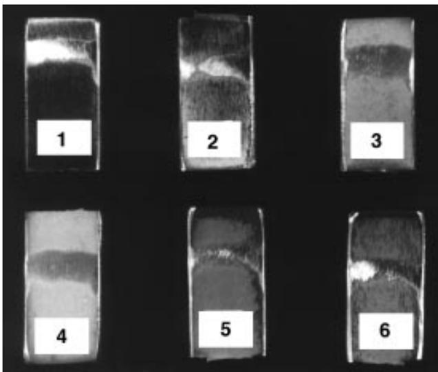
Fig. 5—Views of surfaces of worn Cr-Ni-Al<sub>2</sub>O<sub>3</sub> deposits obtained at current density 7 A/dm<sup>2</sup>; and alumina content of bath at zero (1,2), 125 (3), 50 (4), 187 (5), and 250 (6) g/L; sliding distance 26.4 (1,2) and 30.8 m (3-6).
