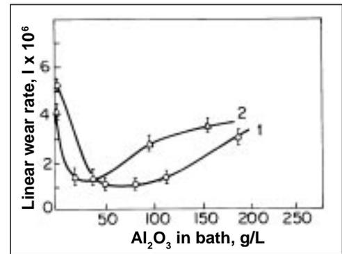
Fig. 4—Linear wear rate of composite Cr-Ni-Al<sub>2</sub>O<sub>3</sub> (1) and Cr-Al<sub>2</sub>O<sub>3</sub> (2) coatings as a function of Al<sub>2</sub>O<sub>3</sub> content of the electrolyte. Current density 7A/dm<sup>2</sup>.
