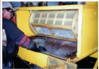
Finished screws are being unloaded from the plating barrel.
