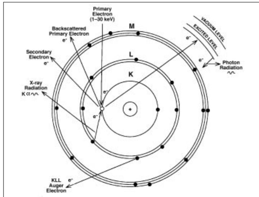
Fig. 1—The interaction of an energetic electron with an atom.
