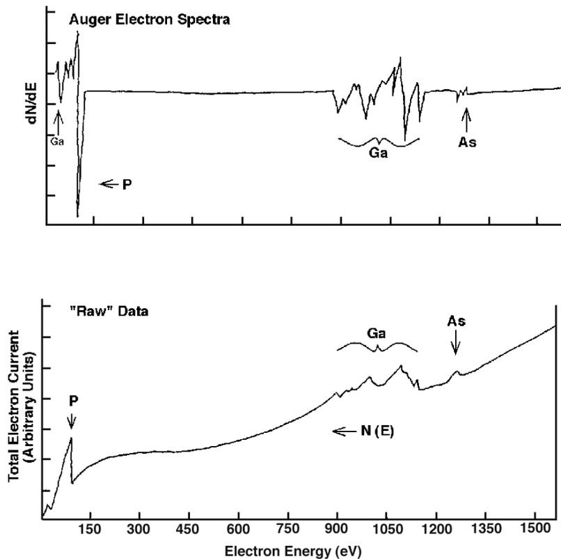
Fig. 2—The electron current collected as a function of the electron energy (raw data) and the Auger electron spectra determined by differentiating the raw data curve.
