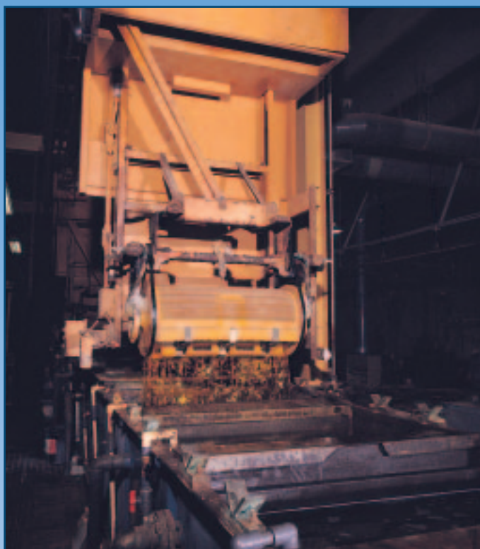
Unique barrel plating techniques, including a patented process for plating drop wires used in the textile industry, are featured at Capsco.
