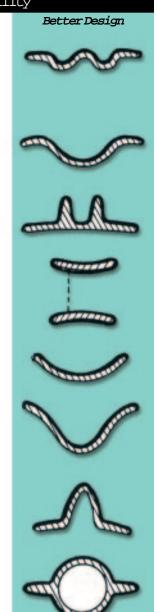
securely on a plating rack with good electrical contact, without masking a significant surface. Many difficult racking problems can be solved by design modification.
