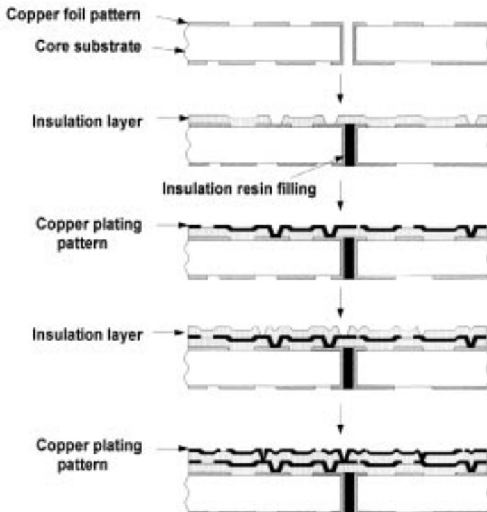
Fig. 1—Preparation of built-up printed circuit boards.
