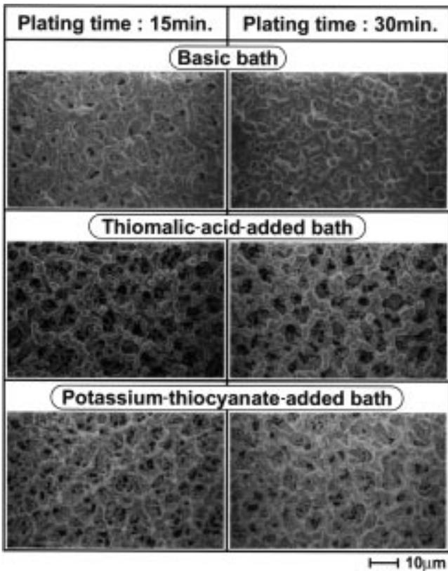
Fig. 7—Surface morphologies of electroless copper on epoxy resin.
