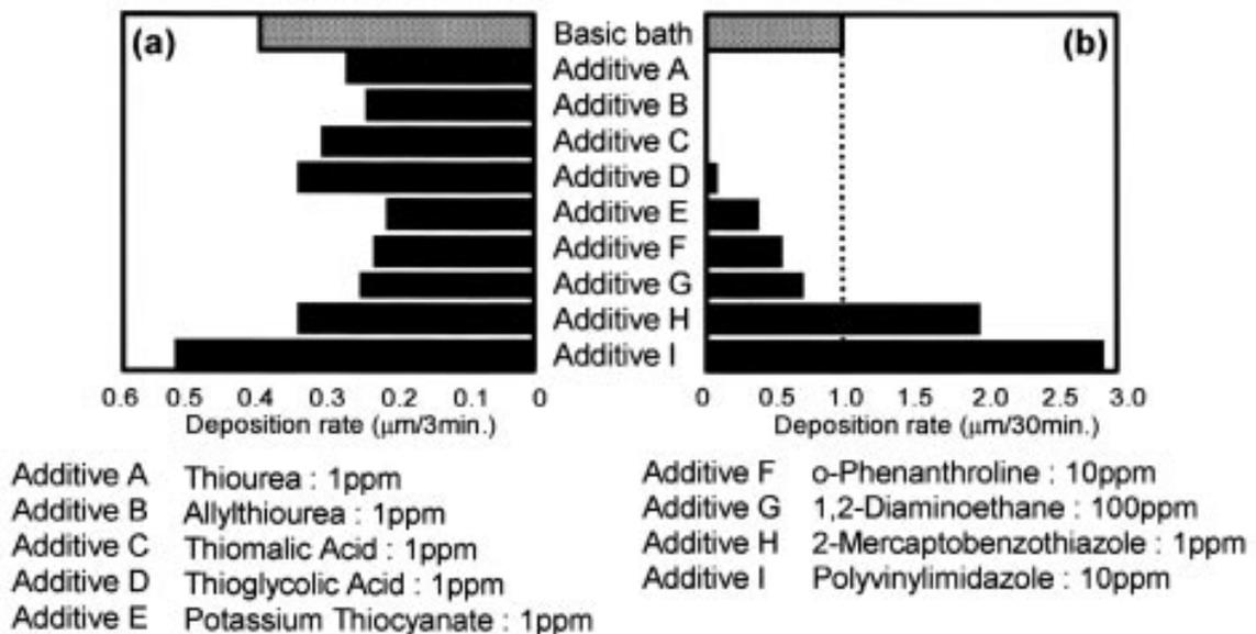
Fig. 6—Effects of various additives on electroless copper plating rate: (a) on palladium catalytic nuclei; (b) on copper.
