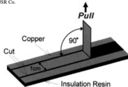
Fig. 2—Peeling test evaluation.
