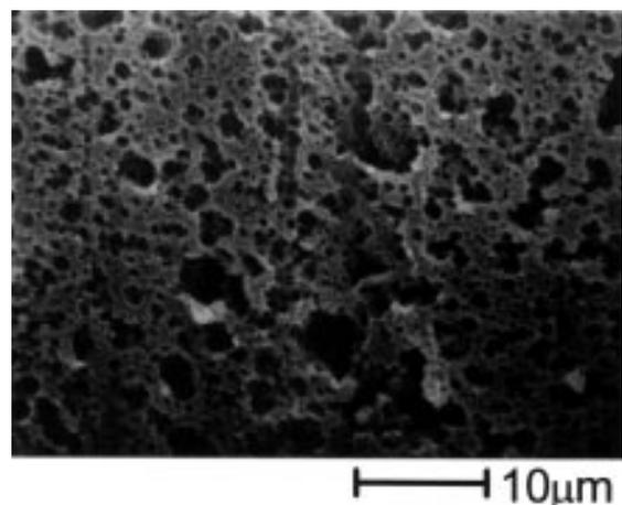
Fig. 3—Surface morphology of LPD resin after etching.
