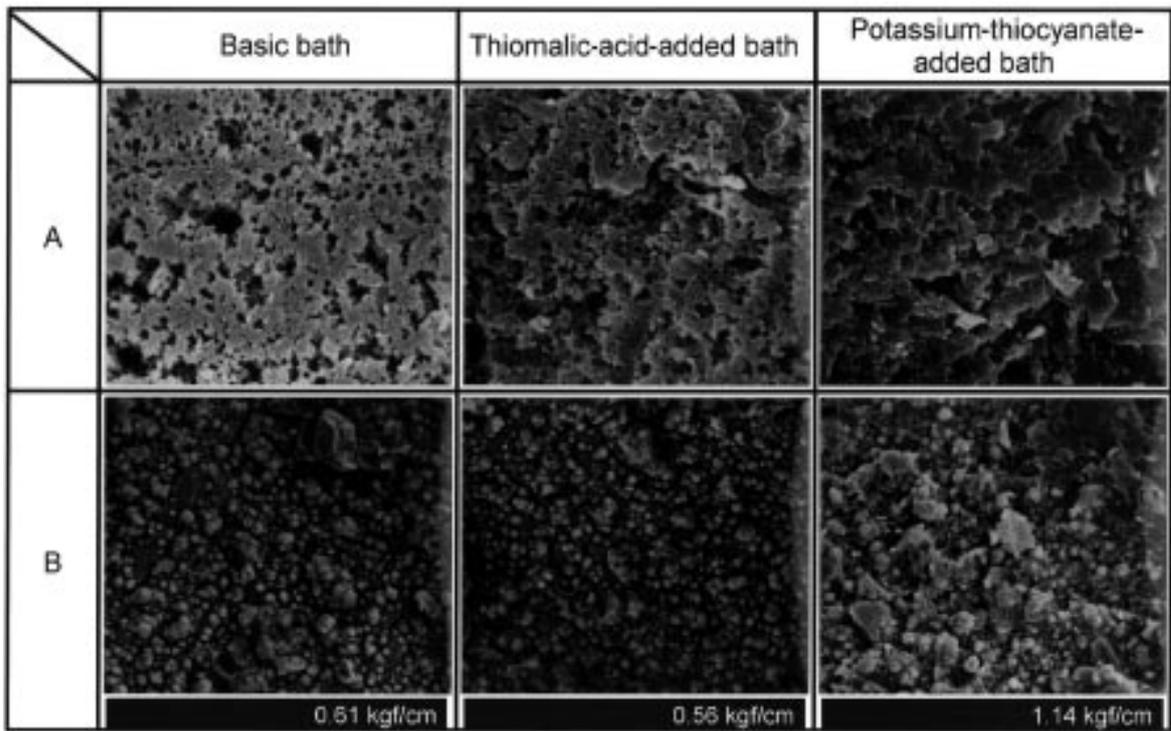
Fig. 9—Surface morphologies after peeling test (LPD resin): (A) resin substrate; (B) backside of peeled copper.
