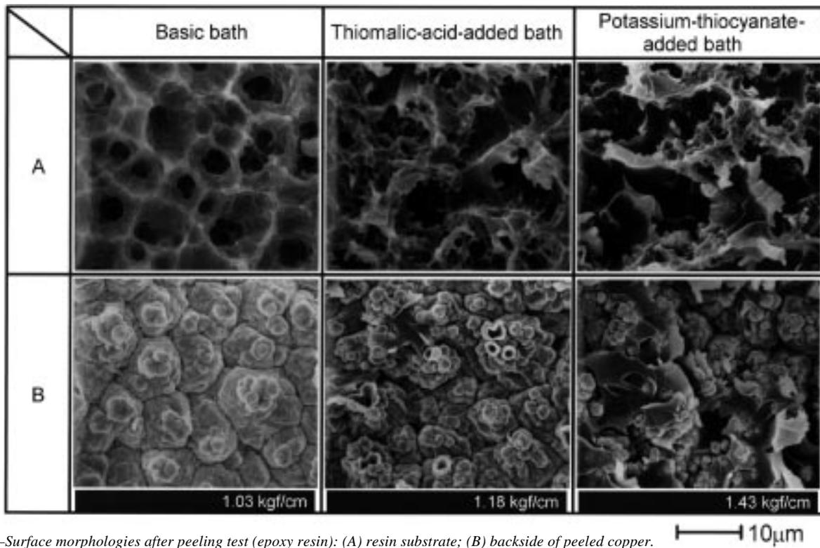
Fig. 8—Surface morphologies after peeling test (epoxy resin): (A) resin substrate; (B) backside of peeled copper.
