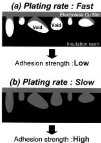
Fig. 4—Schematic model of cross sectional views of electroless Cu plating: (a) with fast plating rate; (b) with slow plating rate.
