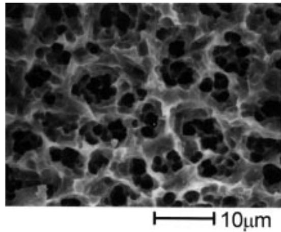
Fig. 5—Surface morphology of epoxy resin after removal of copper.
