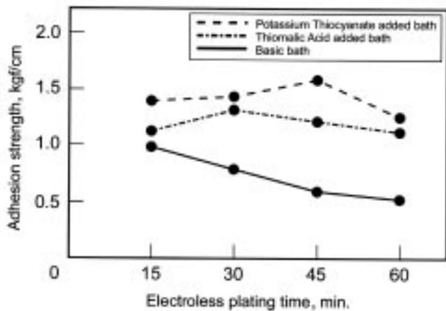
Fig. 11—Influence of electroless copper plating time on adhesion strength (epoxy resin).
