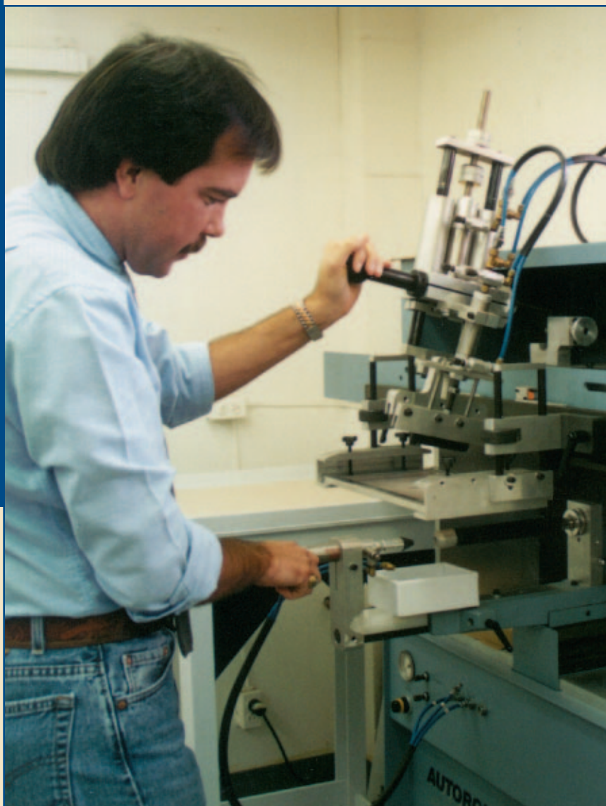
Dan Cunningham, quality control manager, demonstrates the “anofaxing” equipment that is used to place numbers, company or product names, or logos on anodized parts.
