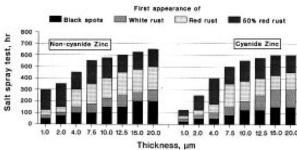
Fig. 4—Influence of plating thickness on salt spray corrosion resistance of zinc deposits with golden yellow passivation.
