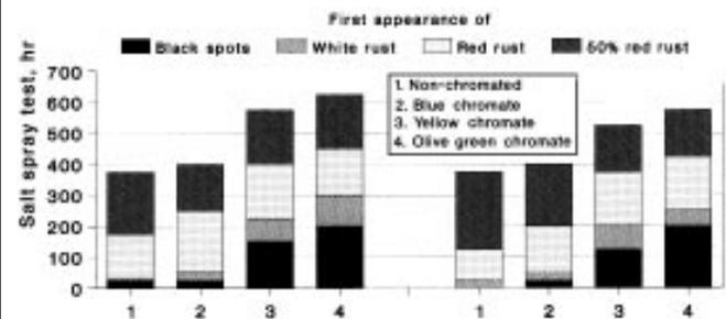
Fig. 5—Salt spray corrosion resistance of zinc deposits with different chromate conversion coatings.
