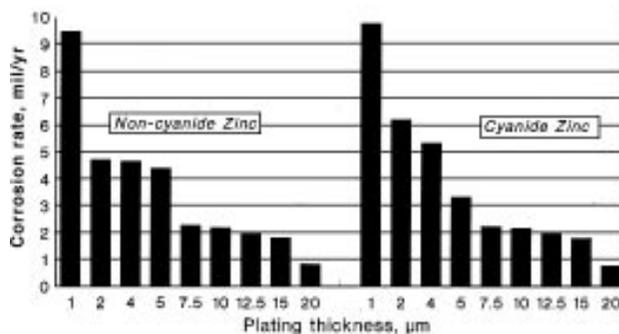
Fig. 2—Influence of plating thickness on corrosion rate of zinc deposits with golden yellow passivation.
