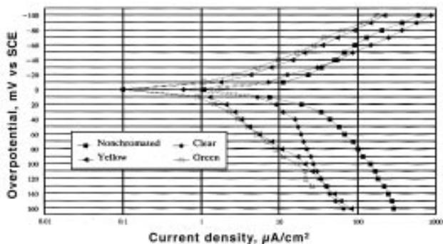
Fig. 1—Typical Tafel polarization curves for non-cyanide zinc deposits (7.5  $\mu$ m) with different chromate conversion coatings.
