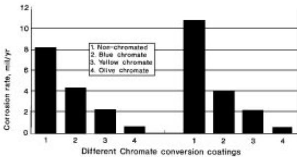
Fig. 3—Influence of chromate conversion coating on corrosion rate of 10- $\mu\text{m}$ -thick zinc deposit.
