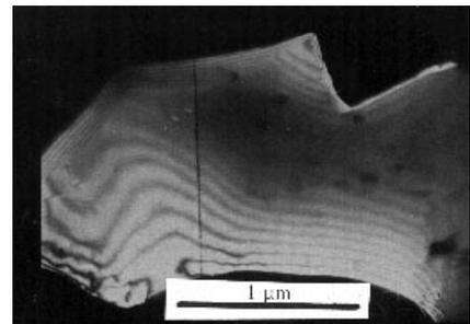
Fig. 3—Transmission electron micrograph showing thickness fringes at the edge of a piece of electroplated nickel.
