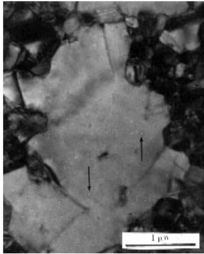
Fig. 5—Transmission electron micrograph obtained by defocusing, showing voids and molecules in a cobalt-hardened gold electrodeposit. (Photograph provided by Dr. Nakahara of Lucent Technologies.)
