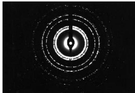
Fig. 7—Electron diffraction pattern of a polycrystalline silver vapor deposit.
