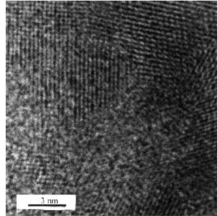
Fig. 1—Transmission electron micrograph showing atom rows in a crystal of yttrium oxide. (Photograph provided by J. Taylor of Stevens Institute.)
