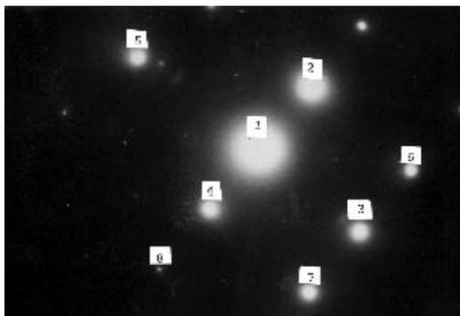
Fig. 6—Electron diffraction pattern of a single grain in a nickel electrodeposit.
