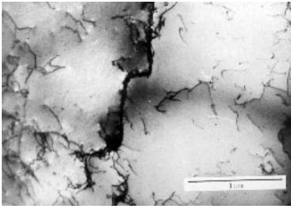
Fig. 4—Transmission electron micrograph showing dislocations in a copper electrodeposit.
