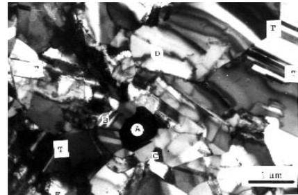
Fig. 2—Transmission electron micrograph of a nickel electrodeposit.
