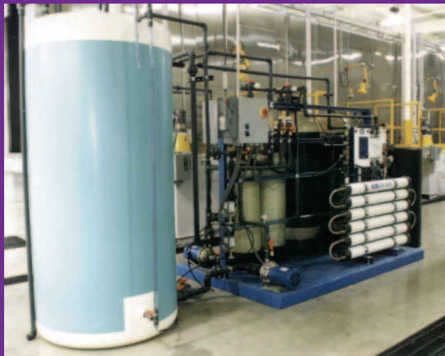
A reverse osmosis system is used to clean contaminated water and provide deionized water for rinsing.
