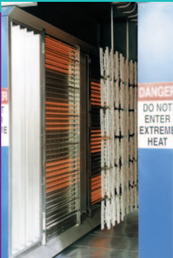
This 216-kilowatt infrared preheat oven “gels” powder before it enters the convection oven for curing.
