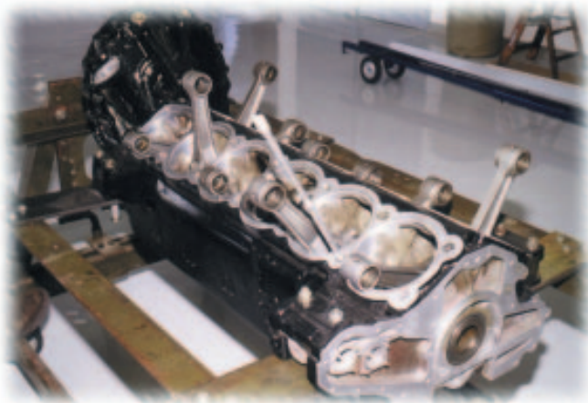
This engine block of a Rolls Royce Merlin V-12 cylinder liquid-cooled motor is part of a current restoration project at Stallion 51 Corporation.
