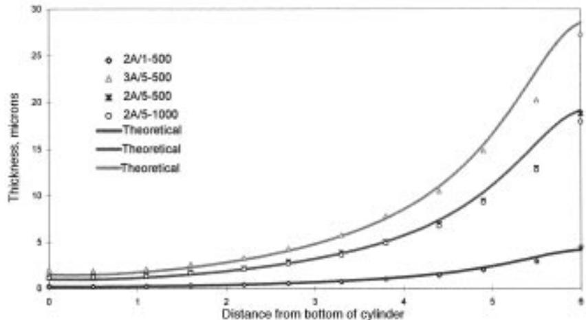
Fig. 1—Coating thickness distribution on the Rotating Cylinder Electrode (RCE). Theoretical values calculated from Eq. (1).
