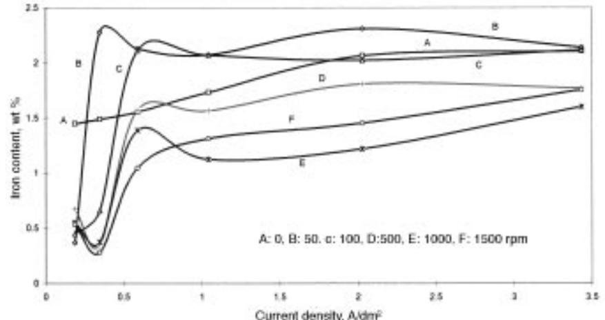
Fig. 2—Iron content (wt pct) in Zn-Fe alloys vs. current density at various RCE rotation speeds for a bath without ammonium chloride.
