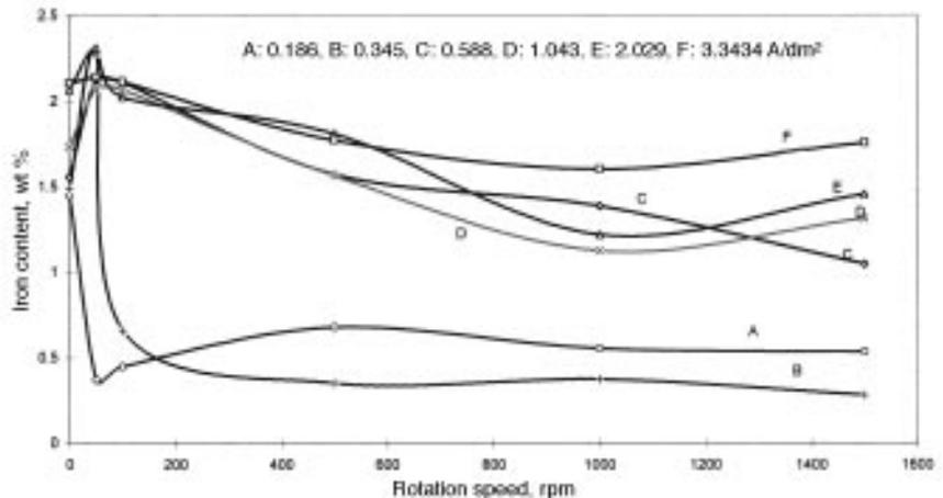
Fig. 6—Iron content (wt pct) in Zn-Fe alloy vs. rotation speed at various current densities for a bath without ammonium chloride.
