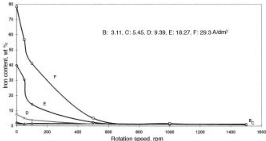
Fig. 7—Iron content (wt pct) in Zn-Fe alloy vs. rotation speed at various current densities for bath without ammonium chloride.
