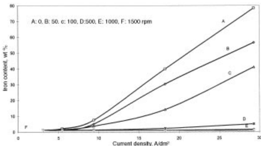
Fig. 3—Iron content (wt pct) in Zn-Fe alloys vs. current density at various RCE rotation speeds for a bath without ammonium chloride.
