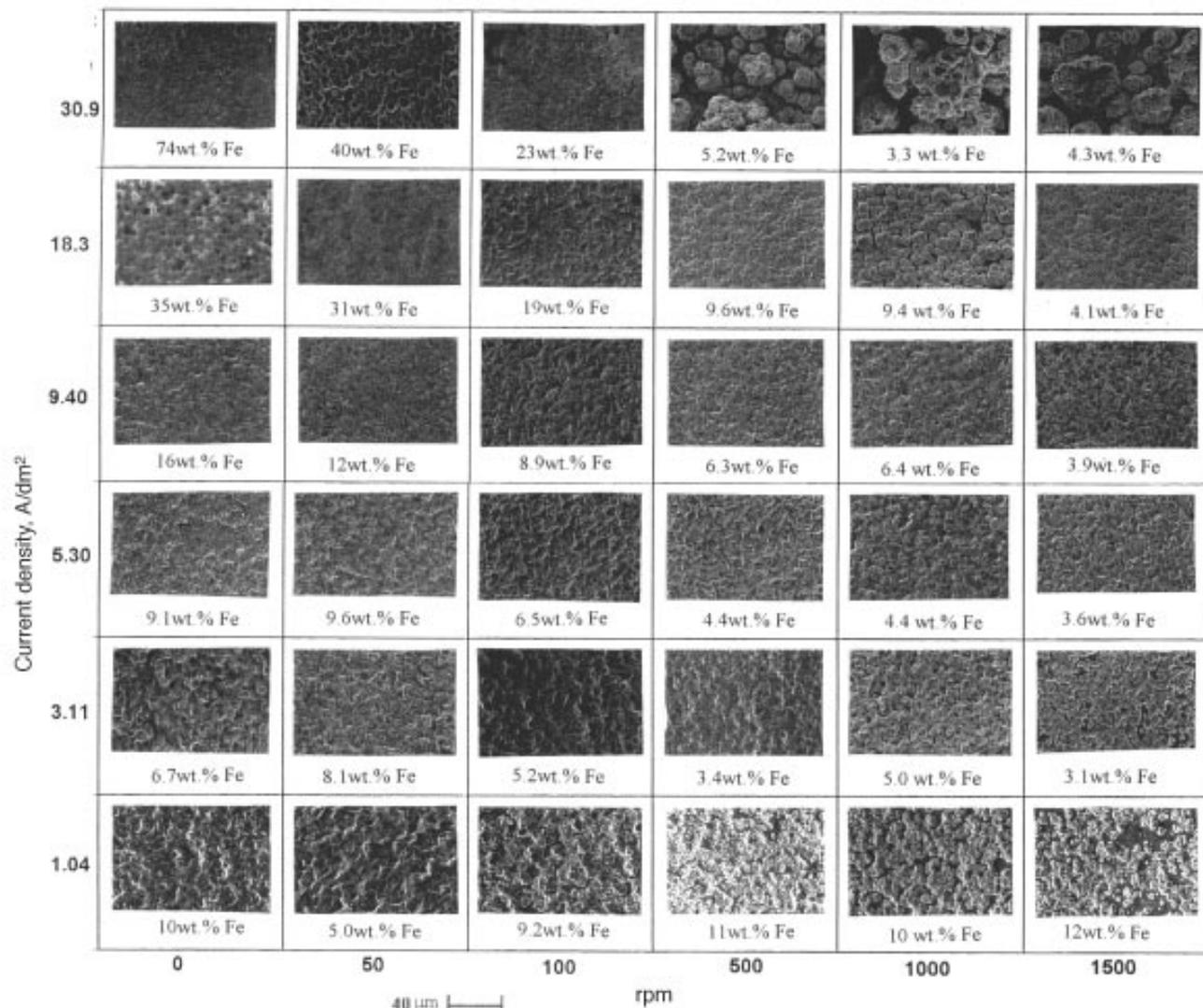
Fig.11—Crystal morphology of Zn-Fe alloy electrodeposits from a solutions with additions of ammonium chloride.
