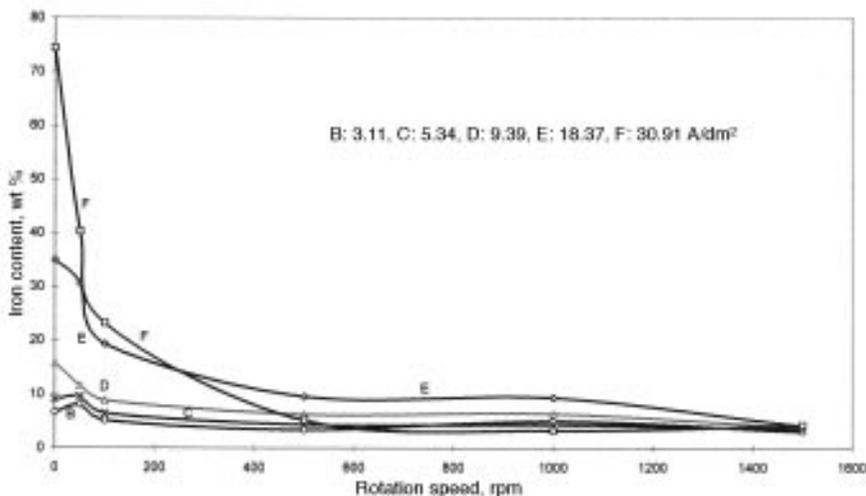
Fig. 9—Iron content (wt pct) in Zn-Fe alloy vs. rotation speed at various current densities for a bath with ammonium chloride.
