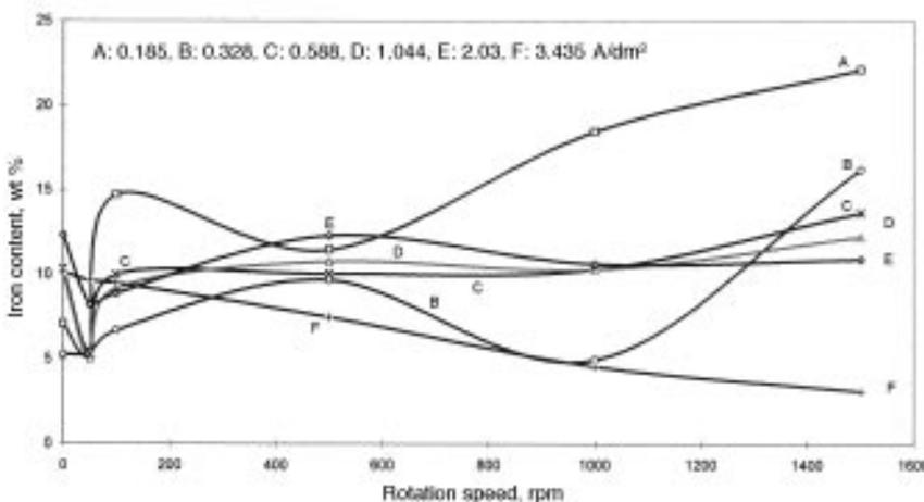
Fig. 8—Iron content (wt pct) in Zn-Fe alloy vs. rotation speed at various current densities for a bath with ammonium chloride.
