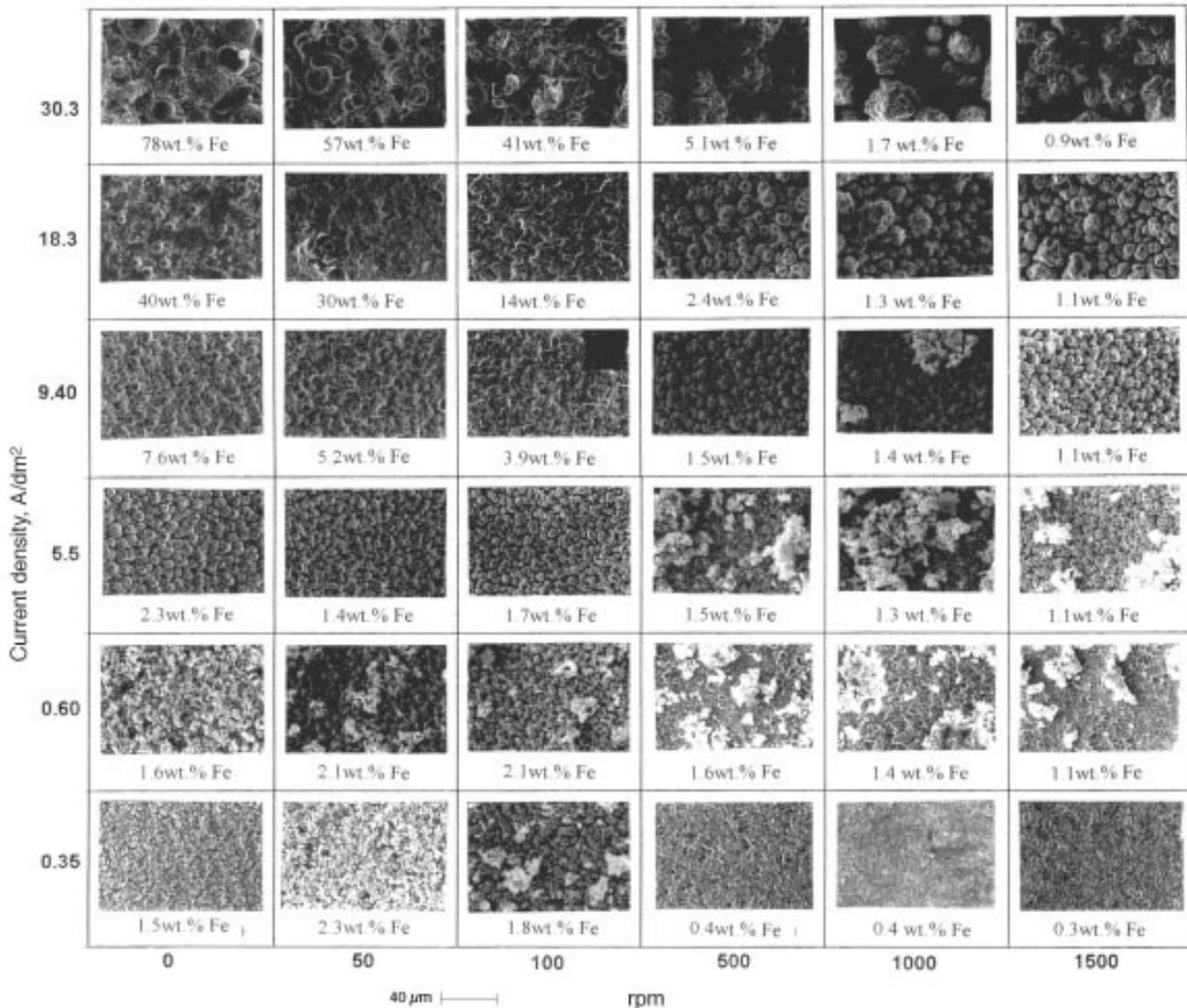
Fig.10—Crystal morphology of Zn-Fe alloy electrodeposits from solutions without ammonium chloride.
