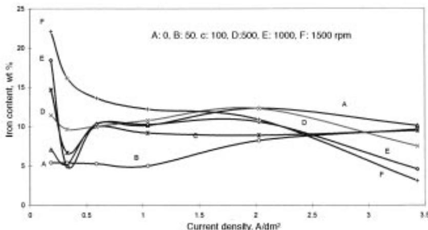
Fig. 4—Iron content (wt pct) in Zn-Fe alloys vs. current density at various RCE rotation speeds for a bath with ammonium chloride.
