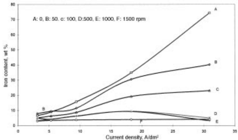
Fig. 5—Iron content (wt pct) in Zn-Fe alloys vs. current density at various RCE rotation speeds for a bath with ammonium chloride.
