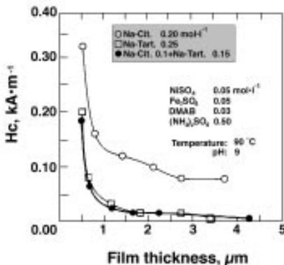
Fig. 1—Effect of film thickness on coercive force.
