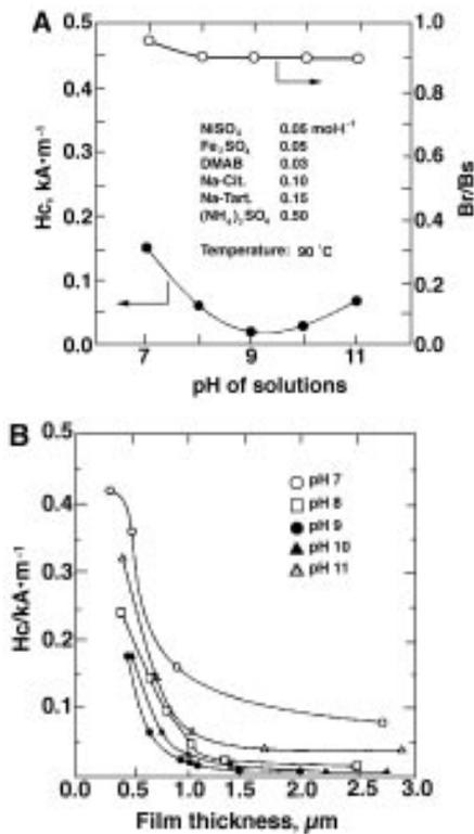
Fig. 3—Effect of solution pH on magnetic properties.
