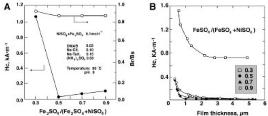
Fig. 2—Effect of metallic salt ratio on magnetic properties.
