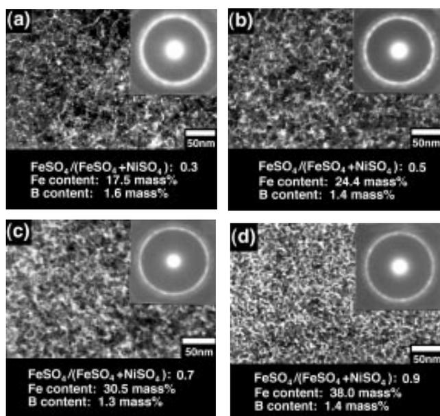
Fig. 6—TEM bright field images of electroless Ni-Fe-B alloy films.
