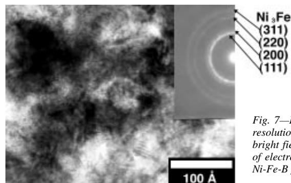
Fig. 7—High-resolution TEM bright field image of electroless Ni-Fe-B film.
