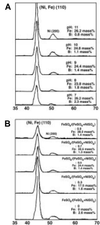
Fig. 5—Changes in X-ray diffraction patterns with (a) metallic salt ratio and (b) solution pH.
