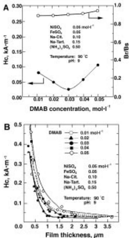
Fig. 4—Effect of DMAB concentration on magnetic properties.
