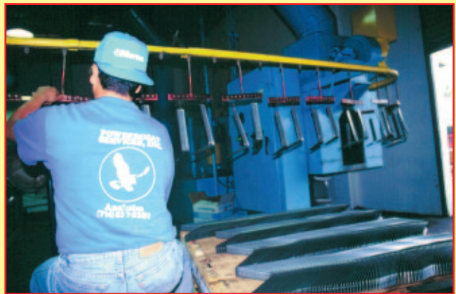
Racking operations for the automatic lines are designed for high-volume production and high-quality results.
