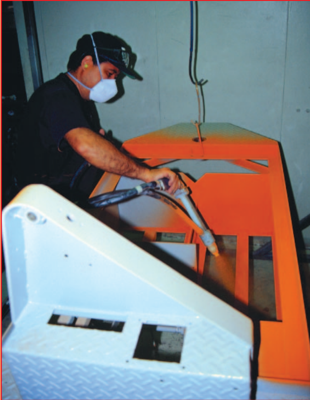
This utility cart frame is one of many items coated by hand application at Powdercoat Services, Inc.
