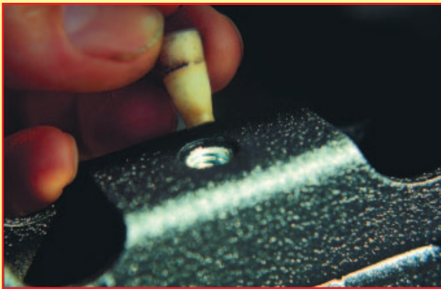
Coatings can be prevented on selected areas by masking before processing.
