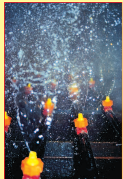
Preparation is an important part of any powder coating operation. This jet spray water wash cleans parts to be processed at Powdercoat Services, Inc.
