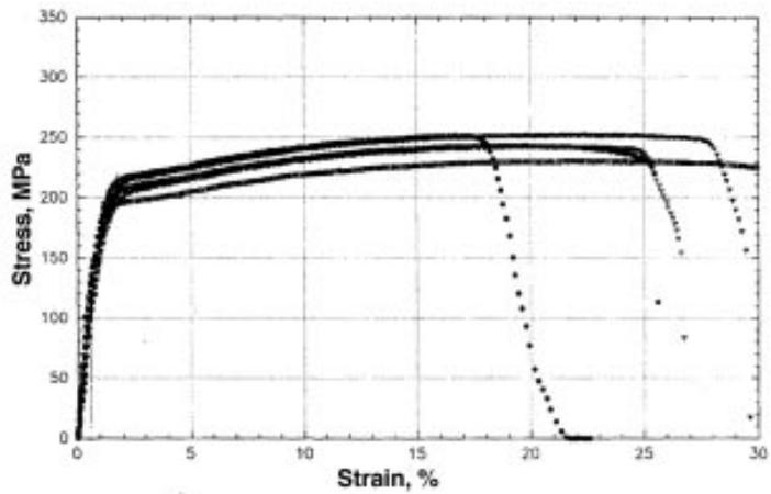
Fig. 1—Nominal stress-strain curves of electrodeposited copper.
