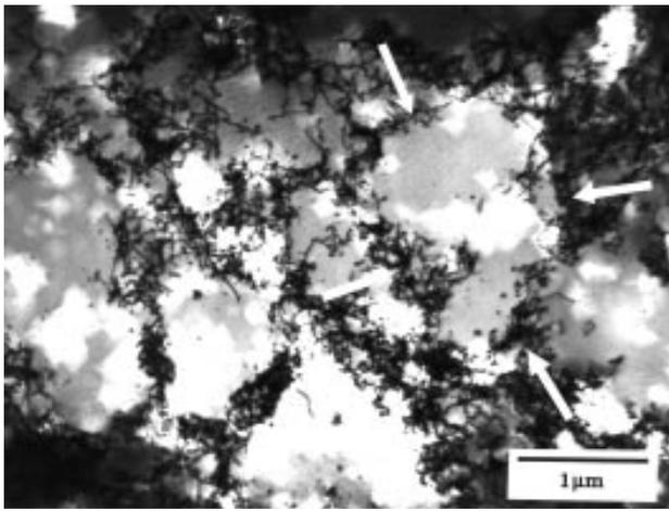
Fig. 2—Transmission electron micrograph showing a dislocation cell structure in electrodeposited copper.
