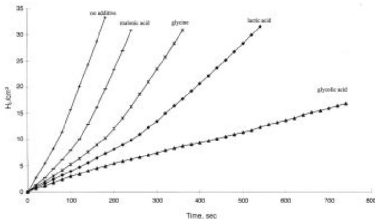
Fig. 4—Effect of different organic compounds on rate of hydrogen evolution at same molar concentration:  $0.88 \text{ mol/dm}^3$ .
