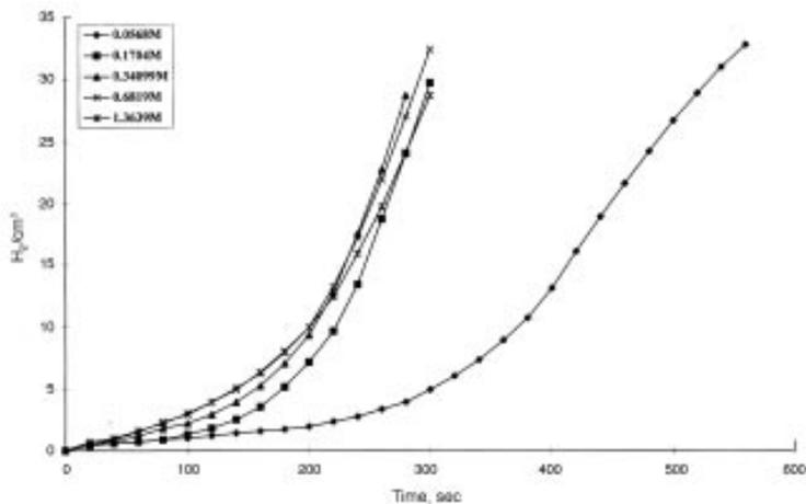
Fig. 2—Effect of hypophosphite concentration on rate of hydrogen evolution.
