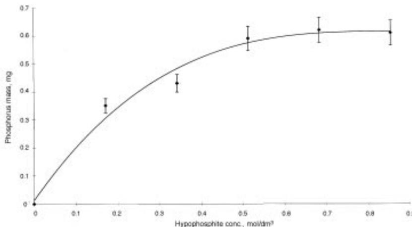
Fig. 1—Effect of hypophosphite concentration on incorporation of phosphorus on nickel catalyst.
