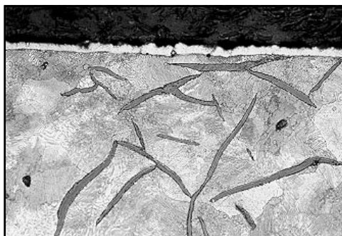
Microscopic cross section, 200X—Surface of cast iron, properly prepared for plating.
