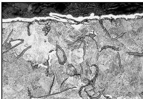
Microscopic cross section, 200X—Surface of cast iron, improperly prepared for plating, resulting in surface roughness and flaking during wear application.
