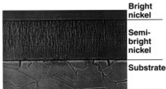
Fig. 10—Cross section of crystallographic structure of a duplex nickel layer.
