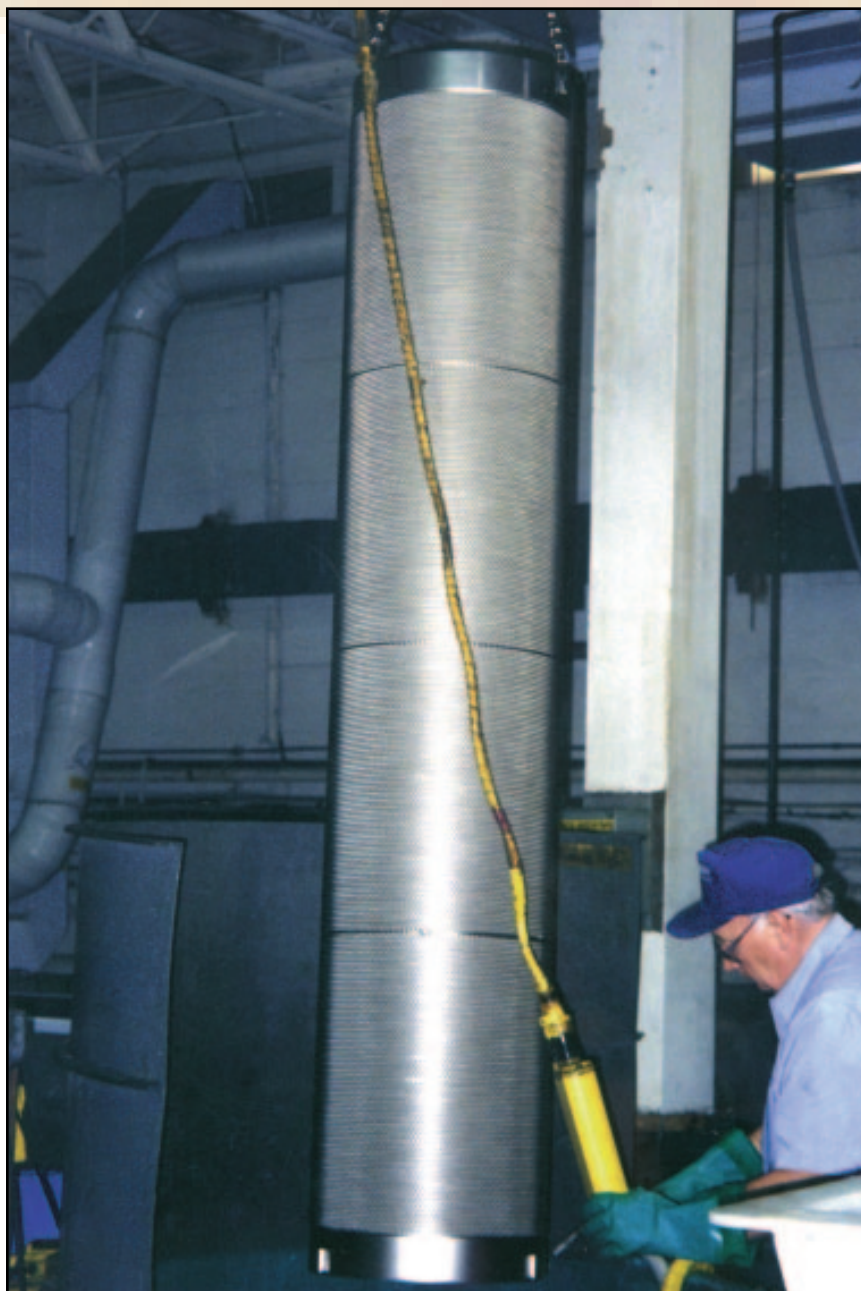
Finishing large parts is a specialty at Twin City. This cylinder, used for removing husks from seeds and grains, receives a high-phosphorus nickel application.
