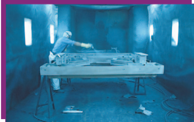
Washex replaced its conventional spray system with a high-volume, low-pressure (HVLP) paint spray system, which has significantly reduced overspray.
