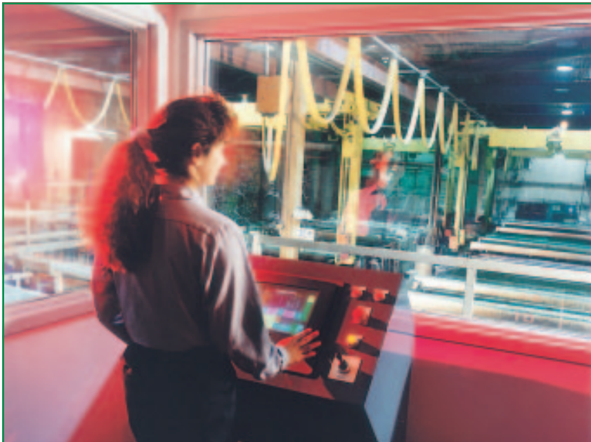
From a separate booth, a system operator oversees the daily work flow using a touch screen interface. A second control screen will allow employees on the plant floor to select the processing steps for each rack they load.
