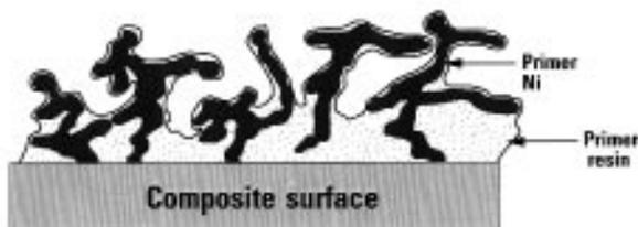
Fig. 1—Sketch illustrating theoretical Ni primer layer structure.
