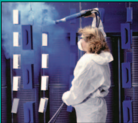
The powder coating area features a five-stage pretreatment line and semi-automatic conveyor. Powder is being sprayed with an electrostatic gun.
