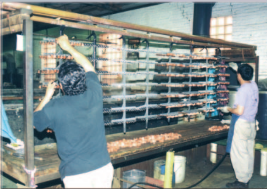
Racks are designed to handle large parts, or a large volume of parts.
