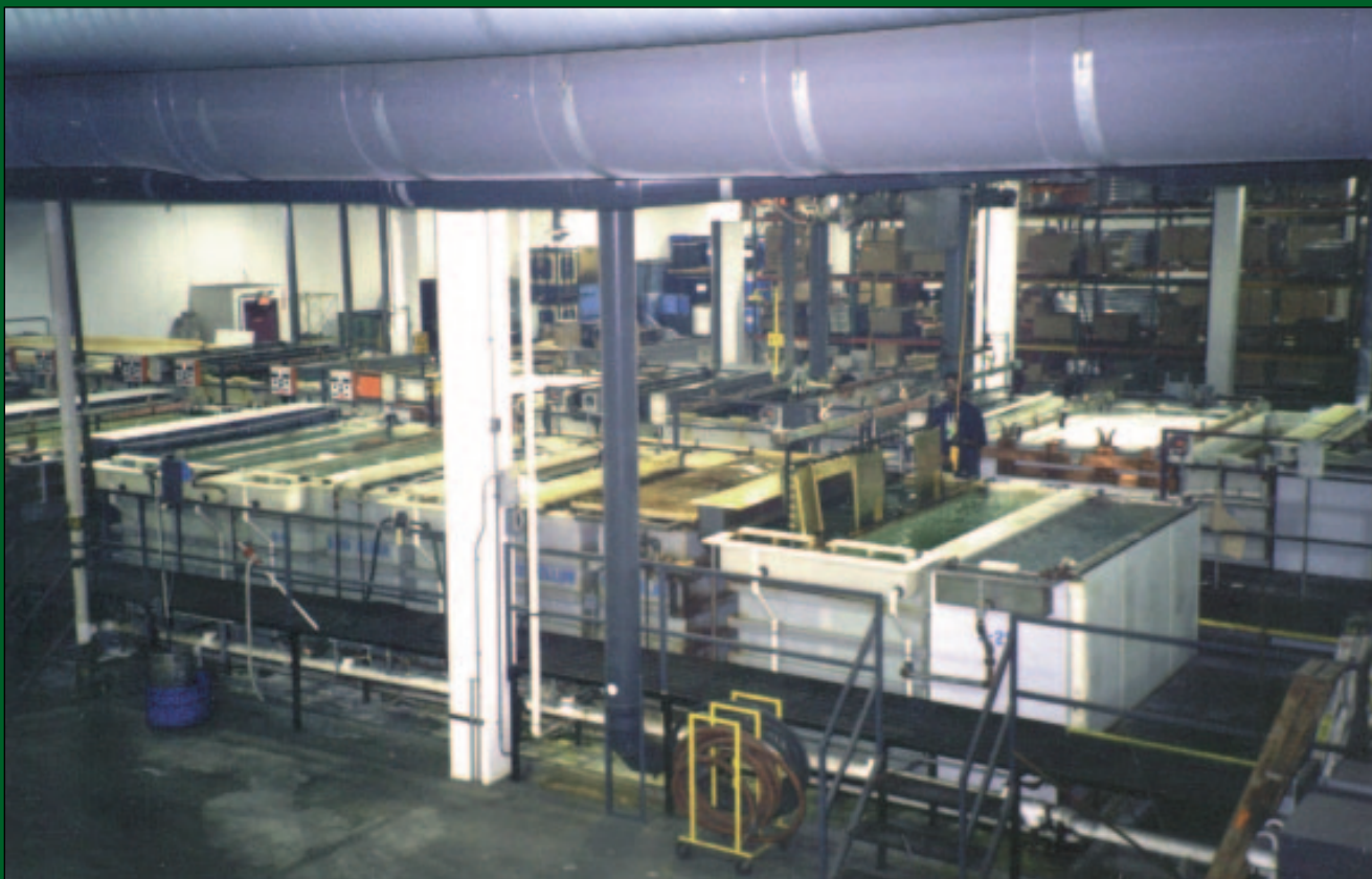
The NiCo facility features automatic, hoist and hand rack plating lines. In the foreground is one of the zinc hoist lines.
