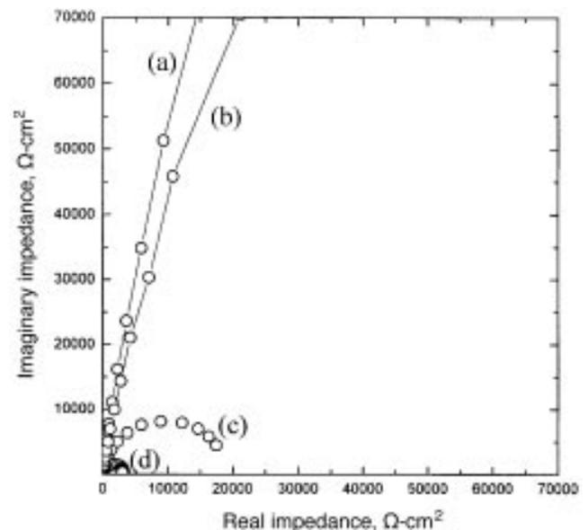
Fig. 2—Nyquist plots for the various layer structures of (a) alloy 42-LF/Pd/Cu/Ni/Pd, (b) Cu-LF/Ni/Pd, (c) alloy 42-LF/Cu/Ni/Pd, (d) alloy 42-LF/Ni/Pd in 3.5 wt pct NaCl solution in the frequency range from 0.1 to 10<sup>5</sup> Hz at the single sinusoidal potential of 5 mV.
