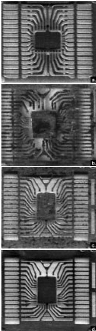
Fig. 1—Surface states for various layers of (a) Cu-LF/Ni/Pd, (b) alloy 42-LF/Ni/Pd, (c) alloy 42-LF/Cu/Ni/Pd, (d) alloy 42-LF/Pd/Cu/Ni/Pd; obtained after salt spray test for 24 hr, by optical microscopy (X3).
