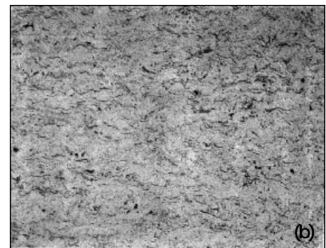
Fig. 2 (a) & (b)—Microstructure of samples that were cross-sectioned, mounted, ground and polished for metallographic examination, showing gray and white lamellar metal oxide phases, surrounded by a nickel-chromium matrix.
