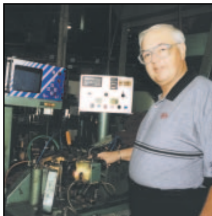
Sorting fasteners for customers represents a separate business at SWD. Here, Dick Delawder shows off a vision sorting machine. Fasteners can be sorted by head diameter, shank length or diameter, cracked heads, partial threads, broken punches, filled recesses and mixed sizes.
