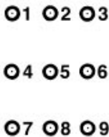
Diagram of sample measurements. Numbers 1-9 designate points of coating thickness measurements.
