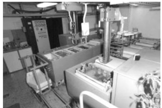
Fig. 2—View of a semi-industrial cell used for the electro-synthesis of Ni-SiC composite coatings. (Photo courtesy of Corroza Engineering, Sofia, Bulgaria)
