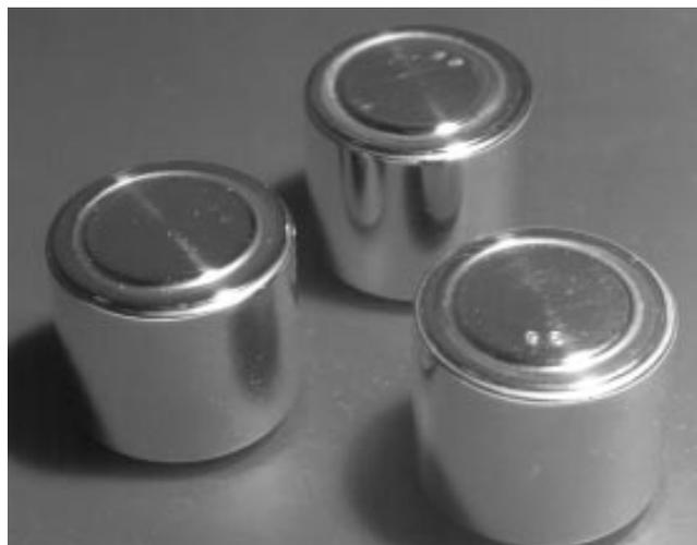
Fig. 6—Punches coated with composite nickel coatings containing β BSC21 C SiC particles (Photo courtesy of Corroza Engineering, Sofia, Bulgaria). These punches were successfully used for forming PVC foils inserted into metal cups of bottles of non-alcoholic drinks.
