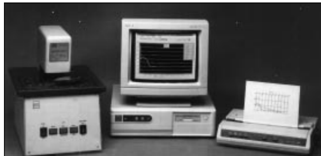
Fig. 2—Computerized sequential electrochemical reduction analysis (SERA) instrument. (Courtesy of ECI Technology, East Rutherford, NJ.)
