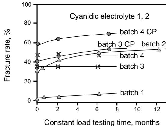
Fig. 8—Fracture dependence on testing time (CP: chemically polished).
