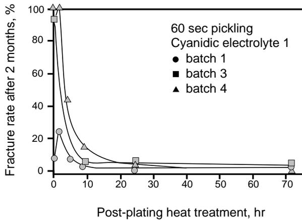
Fig. 3—Fracture dependence on post-plating heat treatment at 220 °C.
