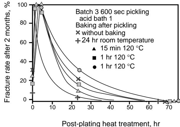
Fig. 6—Fracture dependence on post-plating heat treatment at 220 °C.
