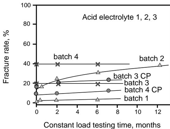
Fig. 7—Fracture dependence on testing time (CP: chemically polished).
