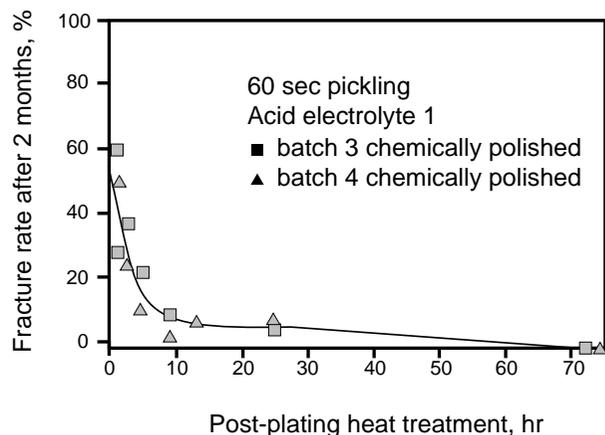
Fig. 2—Fracture dependence on post-plating heat treatment at 220 °C.
