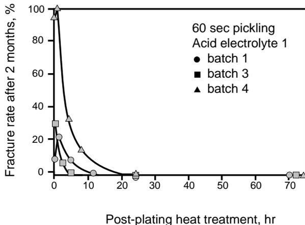
Fig. 1—Fracture dependence on post-plating heat treatment at 220 °C.
