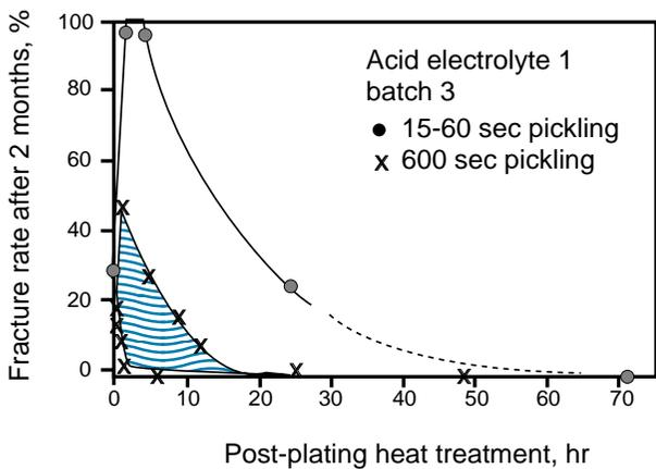
Fig. 5—Fracture dependence on post-plating heat treatment at 220 °C.
