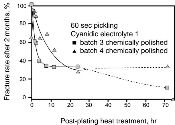
Fig. 4—Fracture dependence on post-plating heat treatment at 220 °C.
