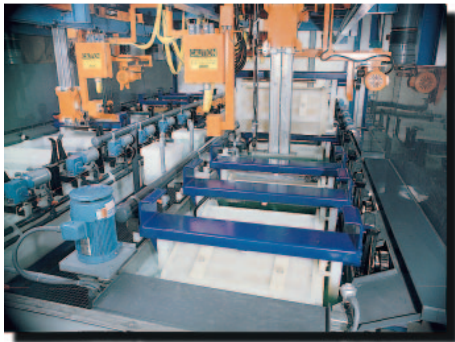
A barrel filled with parts is shown being lowered into the five-cell, 950-gal EN plating tank at FSI.
