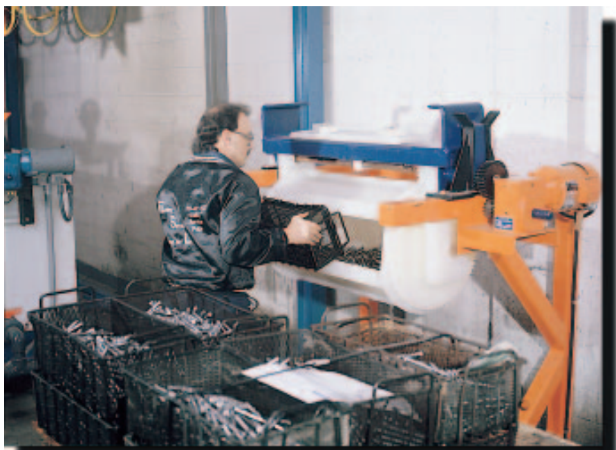
As a specialty jobshop handling small parts, much of the work is handled manually. Here, throttle body shafts are loaded into a barrel that will be automatically moved to the EN plating line.
