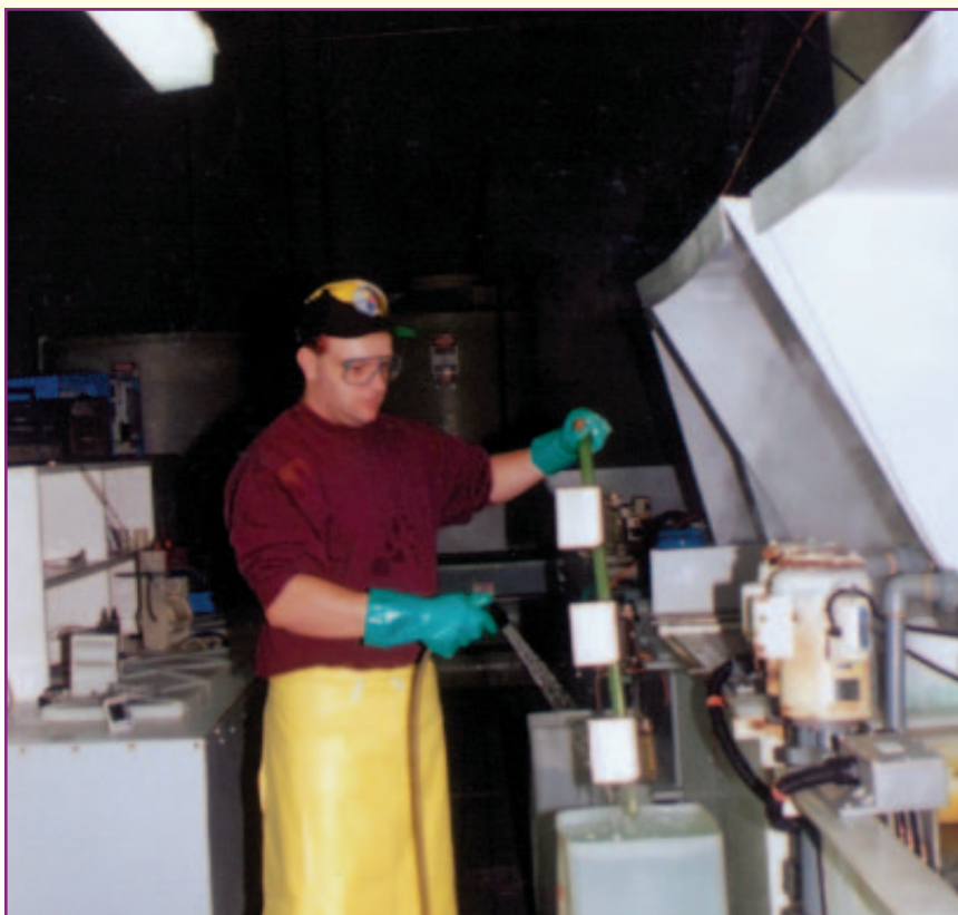
To conserve chemicals and water, there are no flow rinses. Parts are thoroughly sprayed over a tank. When the rinsewater reaches a certain concentration, it is sent through an evaporator.
