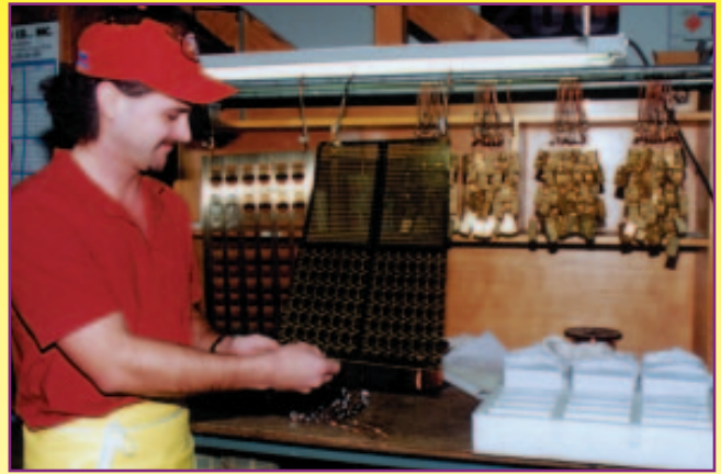
Kreg Avila unracks a variety of parts that have been gold-plated for a number of high-tech clients.
