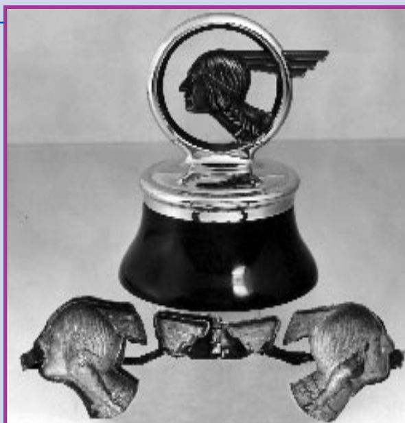
Fig. 1—Radiator cap/hood ornament for a 1930s Pontiac showing the original copper electroform configuration.
