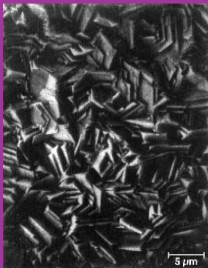
Fig. 6—Surface morphology of a commercial electrogalvanized coating (SEM:3000X).
