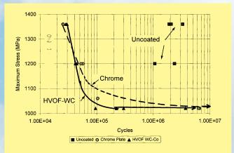
Fig. 4—Axial Fatigue Test Results: R = 0.1,  $K_t = 1.035$  (Courtesy of Messier-Dowty<sup>7</sup>).
