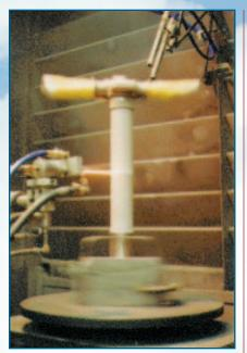
Fig. 6—HVOF spraying of inner cylinder.
