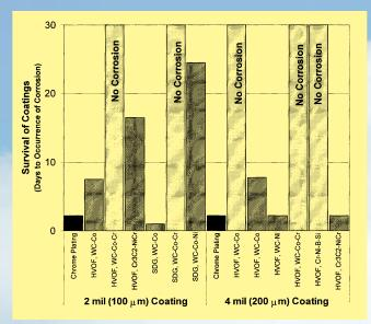
Fig. 3—Summary of Phase I Corrosion Test Results (Photo courtesy of Lufthansa Technik<sup>6</sup>).
