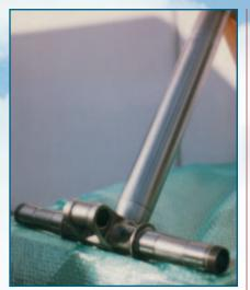
Fig. 2-B737 nose landing gear-inner cylinder.
