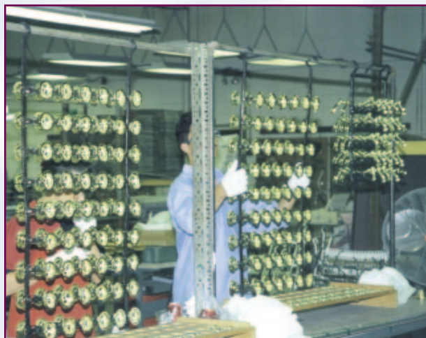
Quality finishing is emphasized in all finishing processes at Artistic Plating. These parts are being racked for powder coating.
