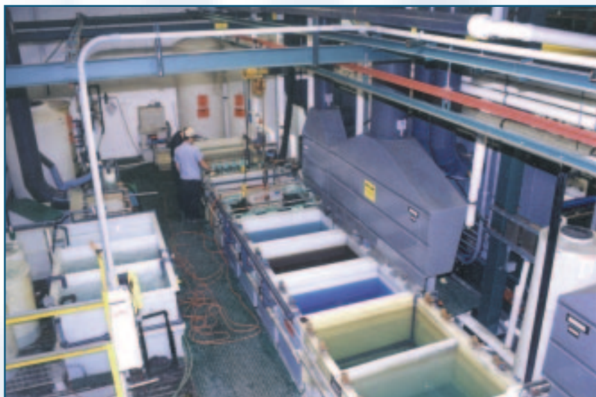
Artistic offers a variety of electroless nickel plating and other electroplating processes, including bright tin, solderable tin, immersion tin, silver, gold, bright nickel, Watts nickel and sulfamate nickel.
