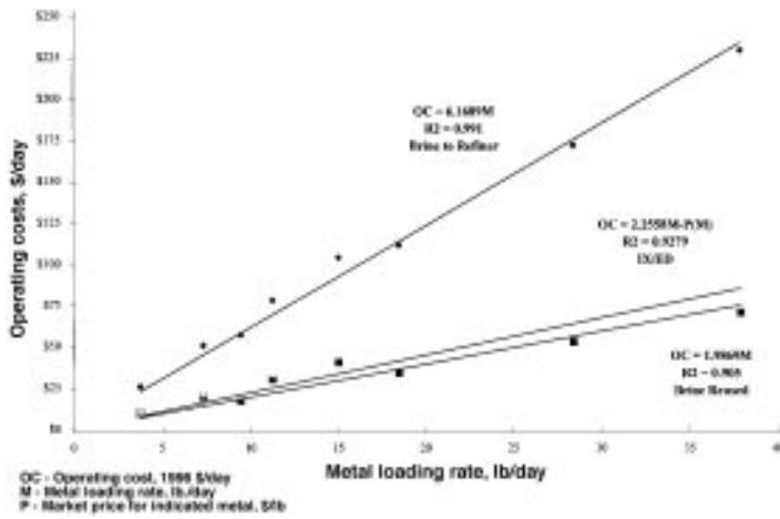
Fig. 8—Copper IX operating costs: Flow rate 38 to 200 gal/min.
