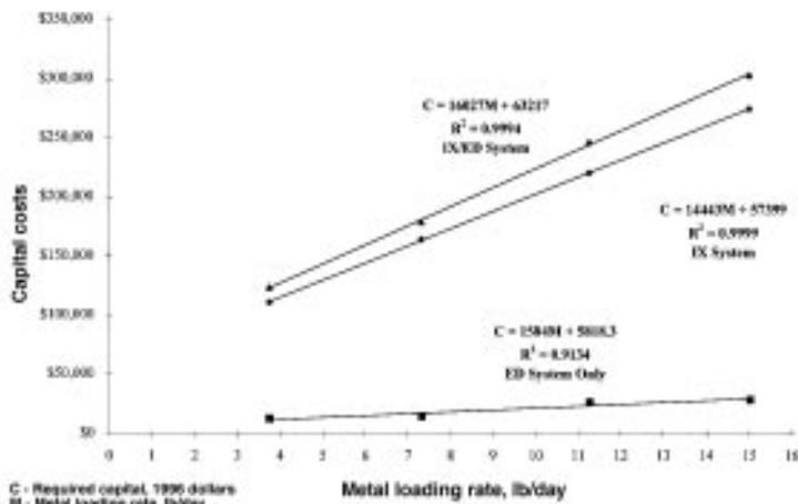
Fig. 5—Ion exchange required capital costs: high-flow, low-concentration, 9-38 gal/min.
