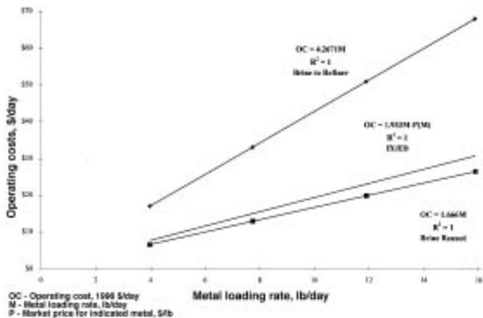
Fig. 9—Nickel IX operating costs: Flow rate 4 to 17 gal/min.
