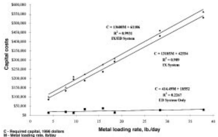
Fig. 4—Ion exchange required capital costs: low-flow, high-concentration, 17-200 gal/min.
