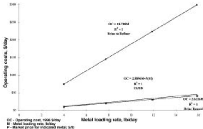
Fig. 10—Nickel IX operating costs: Flow rate 17 to 68 gal/min.
