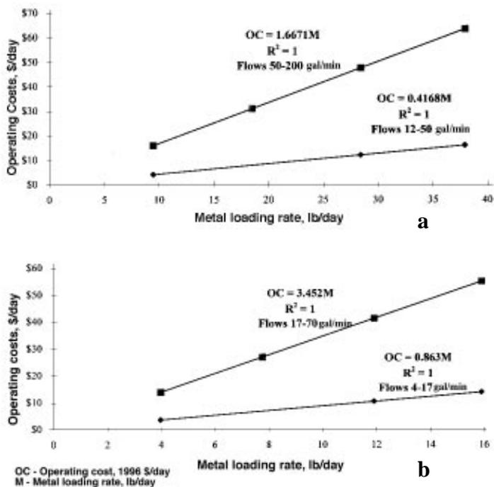
Fig. 12—SP operating costs: (a) copper; (b) nickel.
