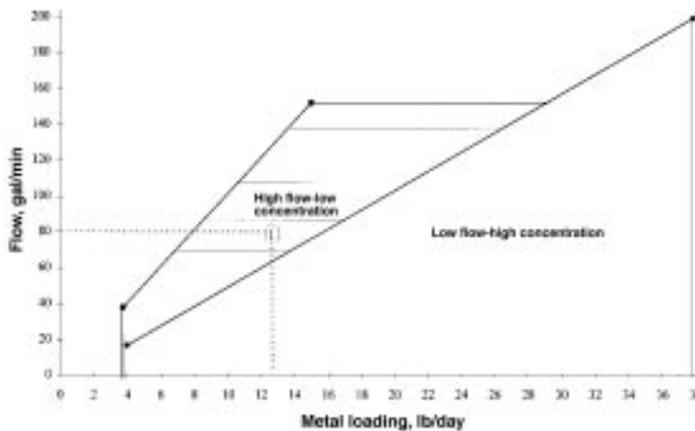
Fig. 2—Operating range for ion exchange systems.
