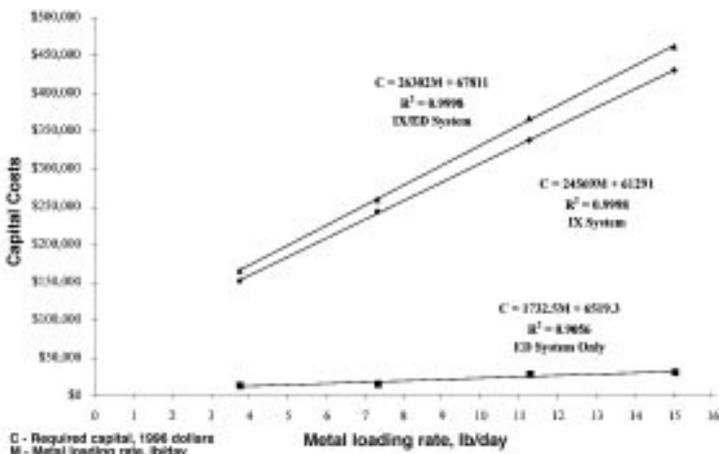
Fig. 6—Ion exchange required capital costs: high-flow, low-concentration, 38-152 gal/min.
