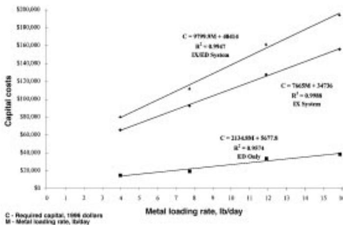
Fig. 3—Ion exchange required capital costs: low-flow, high-concentration, 4-17 gal/min.
