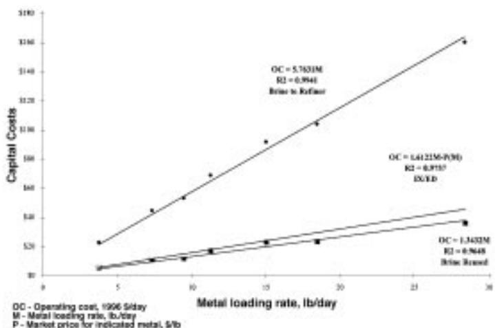
Fig. 7—Copper IX operating costs: flow rate 9.5 to 38 gal/min.
