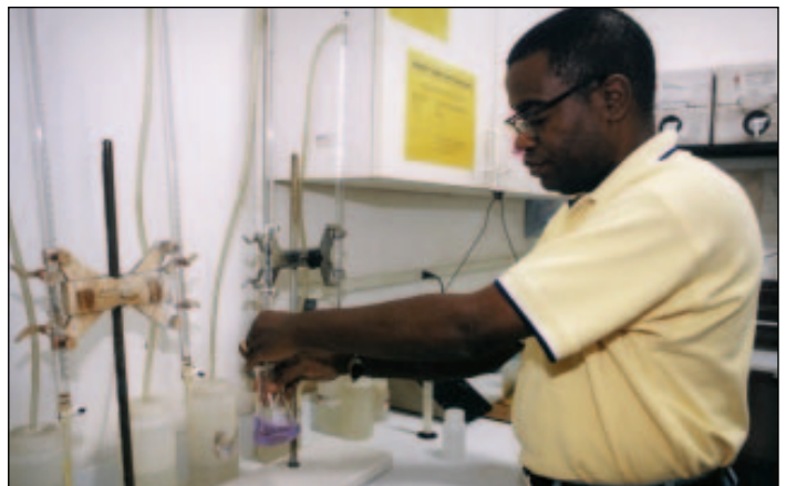
Mark Williams, quality control supervisor, tests a sample from the electro dialysis machine to check nickel metal and orthophosphite levels.
