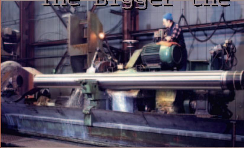
Plated in a single operation, this 25-ft piston rod is being finish-ground in a giant cylindrical grinder.
