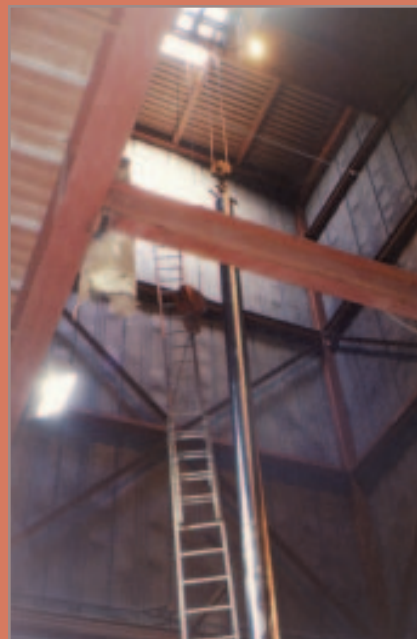
Parts as long as 50 ft can be hoisted into the 60-ft tower and plated in the 30-ft-deep tank below.
