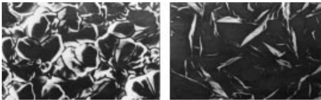
Fig. 6—SEM photomicrographs of tin deposits: (a) from bath A; (b) from Bath B
