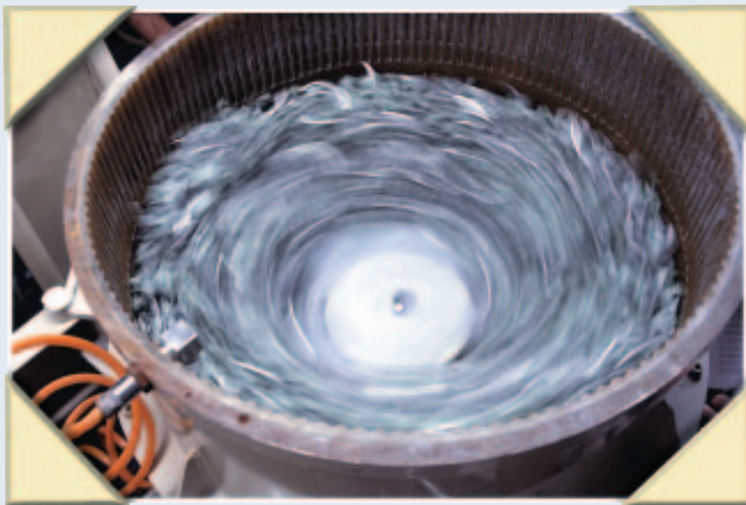
A high-speed rotary finisher performs excellent base metal preparation for matte finishes.
