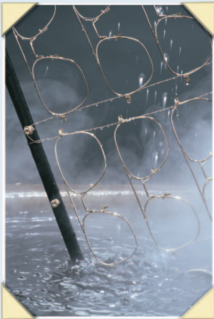
Products such as eyeglass frames that come in direct contact with the skin can use nickel-free processes to meet European regulations.
