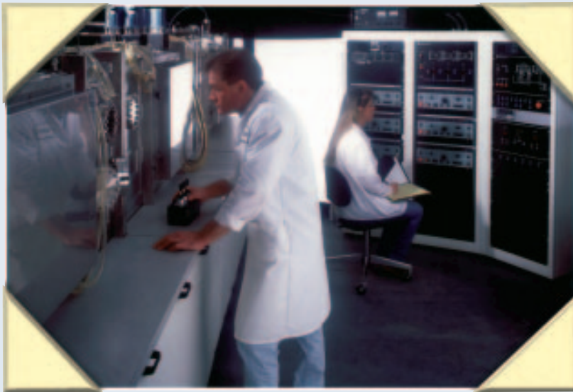
Tanury Industries' in-line PVD (sputtering) system is an environmentally clean process that deposits high-wear, thin, decorative films
