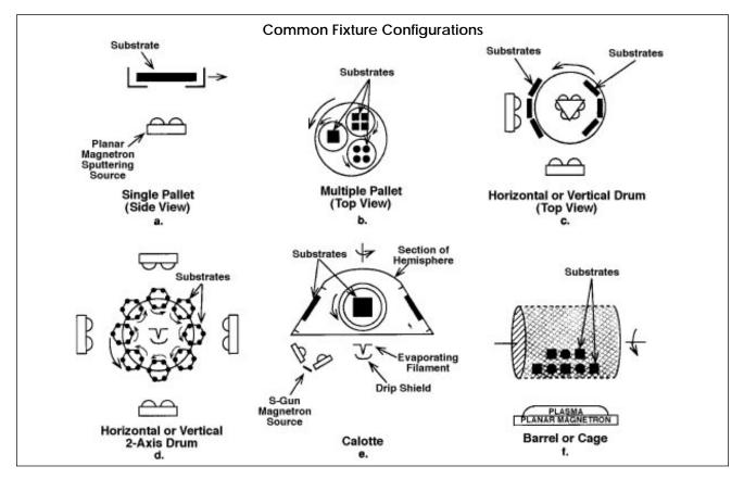
If the fixture is rotating or translating, electrical contact for DC power must be made through a sliding contact. Often this is through the bearings used on the rotating shaft. Wear, galling and seizure of the contacts can be minimized by:
