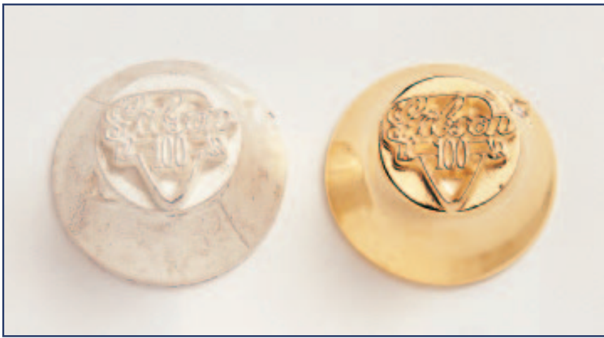
Special control buttons were made depicting "Gibson 100" for use on the Gibson Centennial Collection. This photo shows how buttons appeared before (left) and after plating with 24-karat gold.
