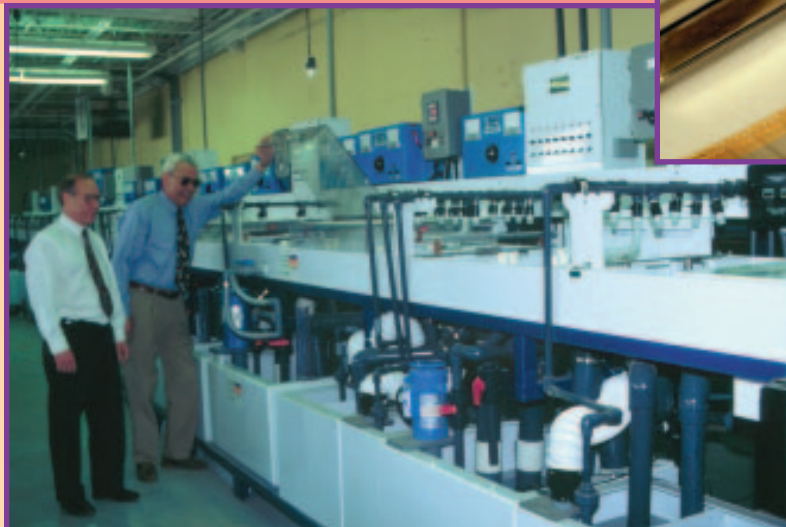
Bruce Anderson and Paul Meyer, Amax owners, are shown here reviewing the installation of a new reel-to-reel plating line with capability of nickel, gold, palladium/nickel and tin/lead plating.
