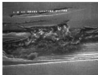
This 1000x SEM photomicrograph represents the same grained 304 stainless steel surface after being mechanically polished to a Buffed No. 8 finish. Note the smeared metal and the depth of the distorted surface profile. While this surface appears very clean and bright to the unaided eye, it remains vulnerable to significant product contamination, as well as ongoing particulation of the imbedded abrasive used in the mechanical polishing and buffing process.
