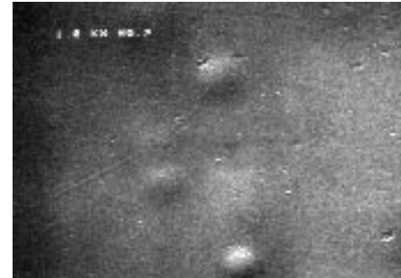
This 1000x SEM photomicrograph represents the same cylinder wall surface after electropolishing. Note the complete absence of grain boundaries and torn metal. Extreme projections in the original surface profile have been rounded off and rendered completely smooth and noncontaminating.
