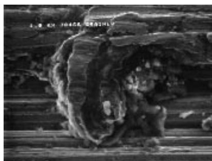
This 1000x SEM photomicrograph represents the surface of grained 304 stainless steel heavy gauge sheet as received from the mill. Note the extreme left-to-right surface striations, combined with the numerous cracks, crevices and torn and distorted metal. This surface offers major contamination potential.
